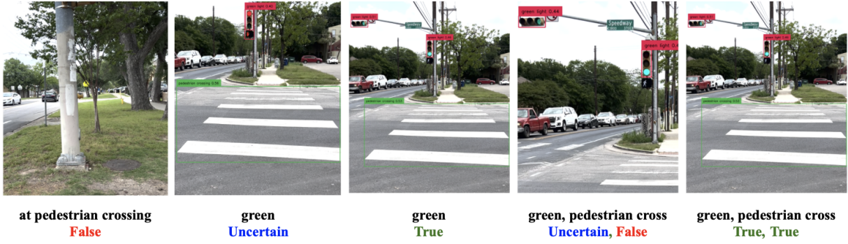
Figure 5: A demonstration Automata2Env implementing control logic under perceptual uncertainties. The figure shows a sequence of observations from the real-world environment, where red and green boxes with confidence scores above are the object detection results from the Grounded-SAM. We use the Grounded-SAM to measure the confidence of image content and evaluate the propositions from the controller. The resulting controller’s state transitions are q_1 \rightarrow q_2 \rightarrow q_2 \rightarrow q_3 \rightarrow q_3 \rightarrow q_4 .
