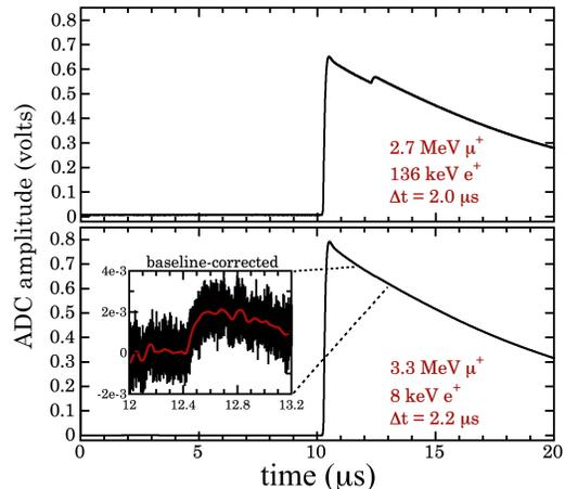
FIG. 3. Two example events. The one in the bottom panel is close to the limit of  $E_{e^+}$  detectability for this run. A red line in the inset shows the denoised trace around the moment of  $e^+$  emission. The value of an in-line capacitor, responsible for the pulse decay visible, was adjusted to provide a compromise between  $E_{e^+}$  threshold and preamplifier reset rate [36].
