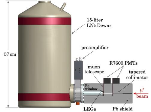
FIG. 1. Schematic of the apparatus. Surface  $\mu^+$  are stopped in a  $0.25 \text{ cm}^3$  n-type germanium detector (LEGe [44]). A trigger is provided by an ultra-thin muon telescope. The device fits on a  $60 \text{ cm} \times 30 \text{ cm}$  tray, weighs less than 50 kg, and is therefore somewhat too small to be described as “table top”.
