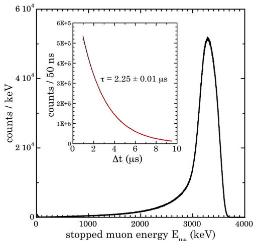
FIG. 2.  $\mu^+$  energy measured by the LEGe detector, degraded from the nominal beam value (4.1 MeV) due to intermediary material traversal. *Inset*: distribution of intervals  $\Delta t$  between  $\mu^+$  and  $e^+$  signals. The small variance between the best-fit value shown and  $\tau_{\mu} = 2.197\ \mu\text{s}$  is traceable to a known systematic affecting  $e^+$  and  $\mu^+$  pulse onset determination differently.
