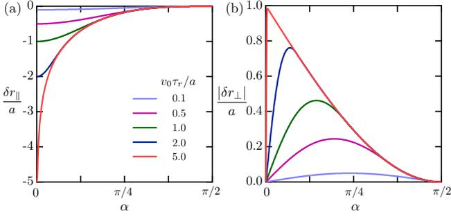
FIG. 6. (a) Longitudinal displacement  $\delta r_{\parallel}/a$  and (b) transverse displacement  $|\delta r_{\perp}|/a$  as functions of incidence angle  $\alpha$ , for different values of  $v_0\tau_r/a$  where  $\tau_r$  is the remaining time in the run after collision.
