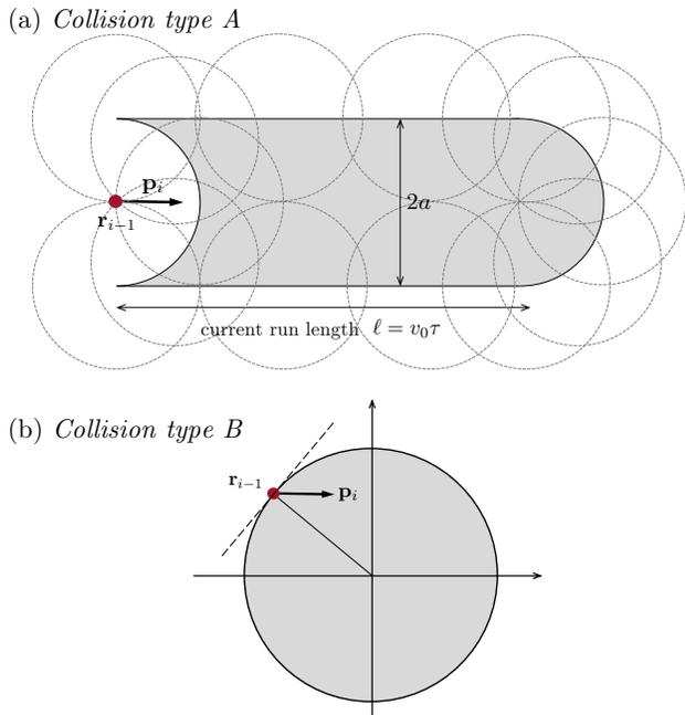
FIG. 3. (a) Collision of type A: for a swimmer initially pointing into the bulk, a collision will occur if the shaded region, of area  $2al$ , contains at least one pillar. Dotted circles show the envelope of pillar positions with which a collision can occur. (b) Collision of type B: a swimmer performing a tumble on the surface of a pillar such that its new orientation points into the pillar will start its new run with a collision.
