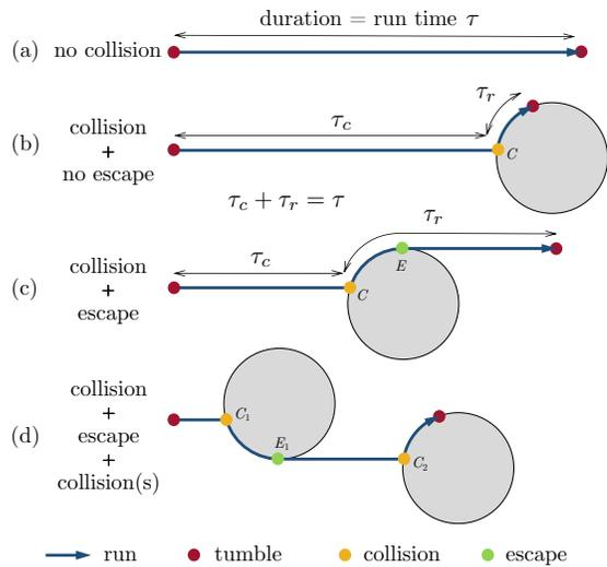
FIG. 2. Types of possible displacements during a single run of total duration  $\tau$ . If the swimmer collides with a pillar (point  $C$ ), it can either escape (point  $E$ ) or end its run on the pillar. The time to collision is  $\tau_c$ , whereas  $\tau_r = \tau - \tau_c$  is the remaining time in the run after collision.
