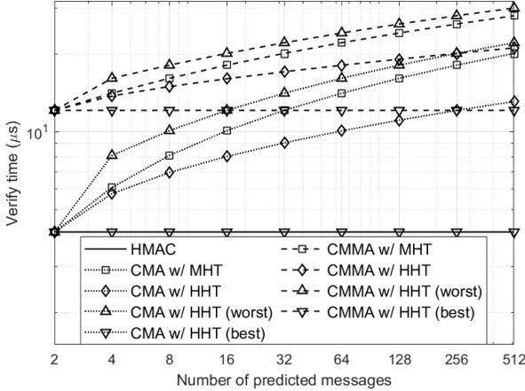
Fig. 7: Verification time over the number of messages. ECDSA is 2500  $\mu\text{s}$ , therefore off the scale. Distribution 3 is assumed.
