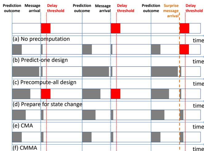
Fig. 2: Processing loads and packet delays under different designs. The scaling does not represent true values.
