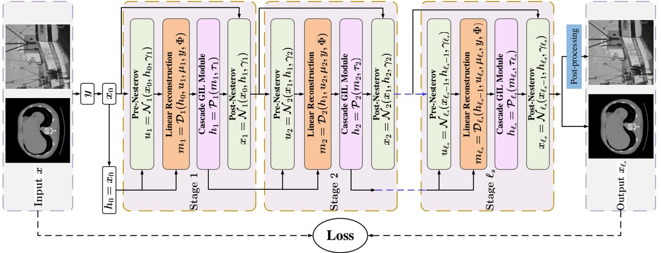
Fig. 1. The overall architecture of our Nest-DGIL network. It consists of four main modules, i.e. linear reconstruction module  $\mathcal{D}_k$ , cascade geometric incremental learning module  $\mathcal{P}_k$ , Nesterov acceleration module  $\mathcal{N}_k$  and post-processing module.
