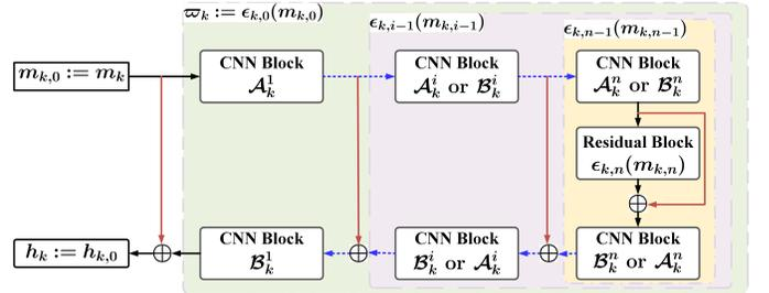
Fig. 3. Cascade GIL module  $\mathbf{h}_k = \mathcal{P}_k(\mathbf{m}_k, \theta_k) = \mathbf{m}_k + \varpi_k$  and geometric incremental component  $\varpi_k$ , where the module shares same parameter  $\mathcal{A}_k^i$  and  $\mathcal{B}_k^i$  in each  $\varpi_{k,i}$ .
