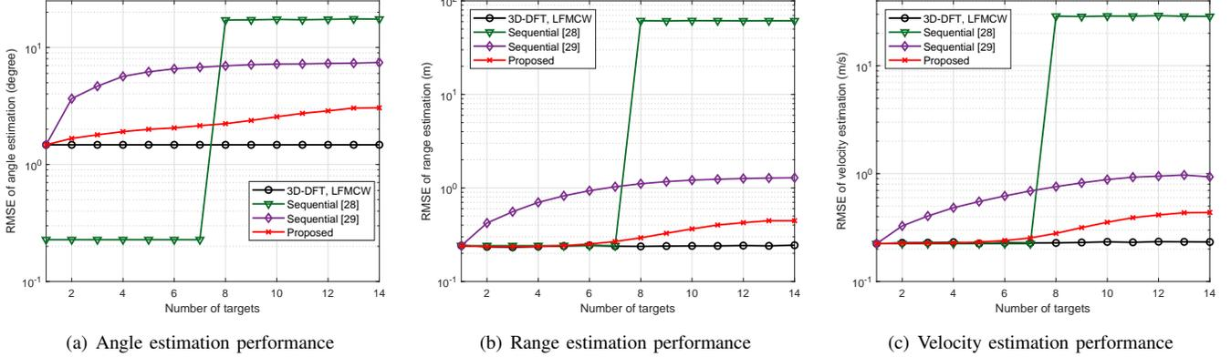
Fig. 7: Estimation performance versus the number of targets,  $M_{\text{TX}} = 8$ .
