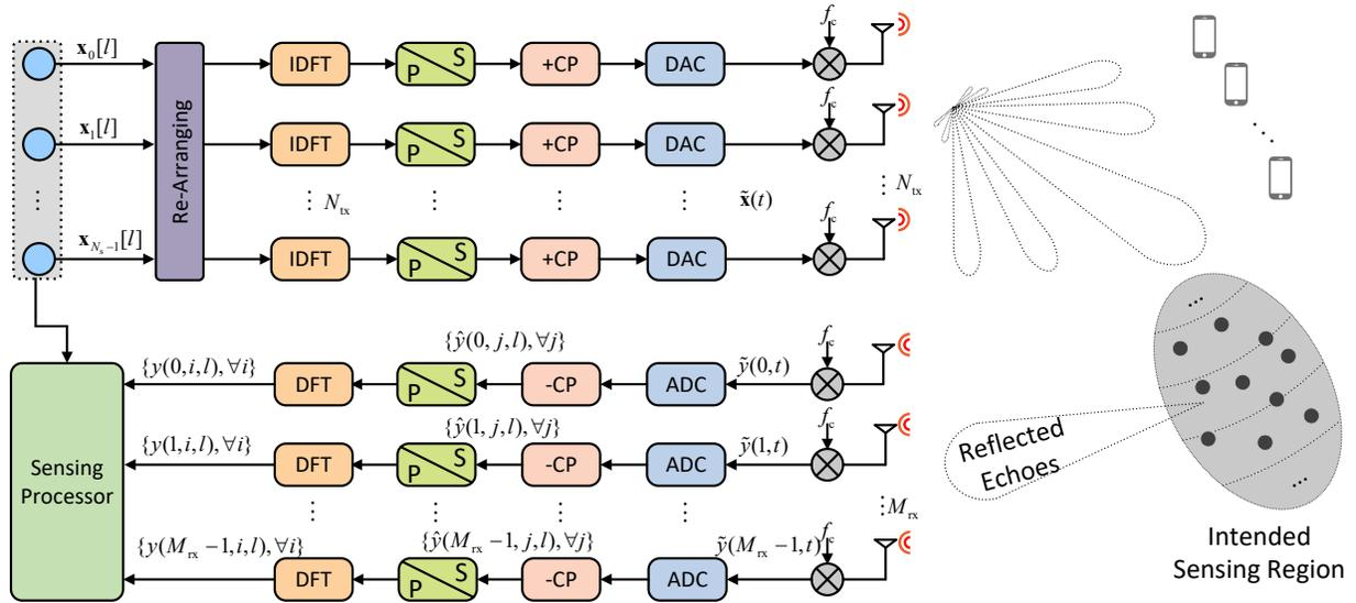
Fig. 1: The considered MIMO-OFDM ISAC system.
