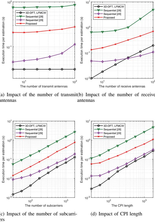
Fig. 6: Execution time per estimation versus the number of transmit antennas, receive antennas, subcarriers, and CPI length.
