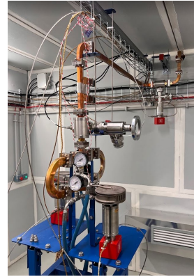
Figure 8 The 3D printed Titanium spiral load setup for the RF high power test at TEX.
