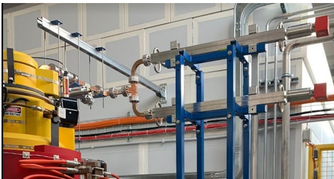
Figure 7 Stainless steel RF load test setup at TEX.
