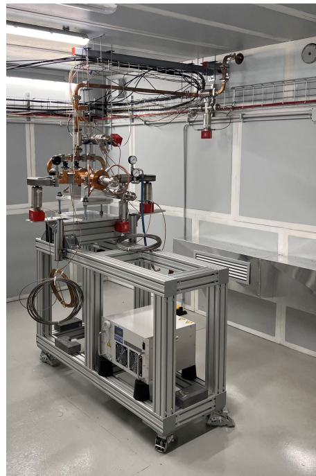
Figure 9 The T24 CLIC accelerating structure, connected with Titanium spiral loads setup ready to be tested in RF high power at TEX.
