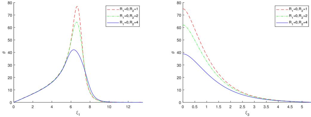
Figure 10: Top surface temperatures in the  $\xi_1$ -direction(left) and temperatures in the  $\xi_3$ -direction(right) of the medium subjected to different sizes of circular laser beams under  $K_\tau = 1$ .
