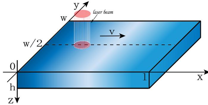
Figure 1: Schematic diagram of the three-dimensional medium with a moving laser beam.
