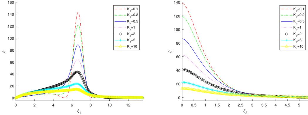
Figure 8: Top surface temperatures in the  $\xi_1$ -direction(left) and temperatures in the  $\xi_3$ -direction(right) of the medium subjected to a circular laser beam under different  $K_\tau$ .
