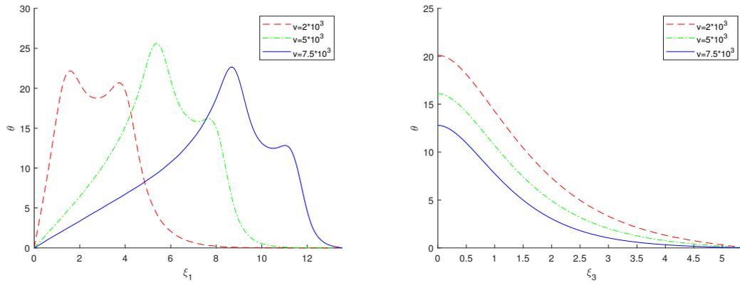
Figure 13: Top surface temperatures in the  $\xi_1$ -direction(left) and temperatures in the  $\xi_3$ -direction(right) of the medium subjected to an annular laser beam with different moving speeds under  $K_\tau = 1$ .
