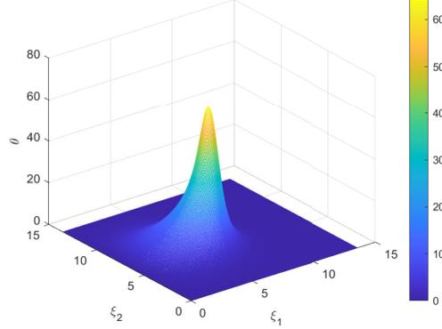
(a) The 3D temperature distribution on the surface of the medium.
