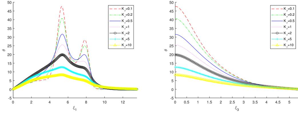
Figure 9: Top surface temperatures in the  $\xi_1$ -direction(left) and temperatures in the  $\xi_3$ -direction(right) of the medium subjected to an annular laser beam under different  $K_\tau$ .
