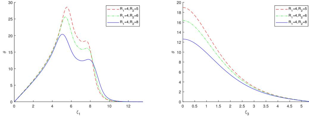
Figure 11: Top surface temperatures in the  $\xi_1$ -direction(left) and temperatures in the  $\xi_3$ -direction(right) of the medium subjected to different sizes of annular laser beams under  $K_\tau = 1$ .
