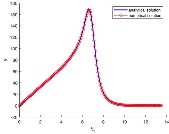
Figure 3: Comparison of analytical and numerical solutions for the top surface temperature distribution on  $\xi_2 = W/2$ .
