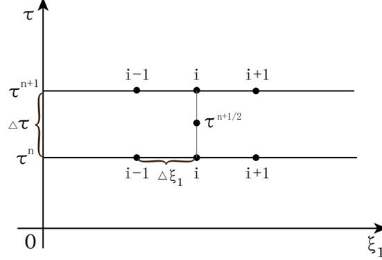
Figure 2: A grid computing model with implicit finite difference in the  $\xi_1$ -direction.
