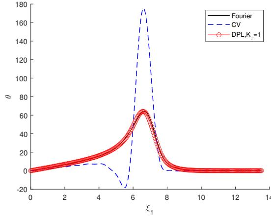
Figure 4: Top surface temperatures on  $\xi_2 = W/2$  with a circular laser beam under different models.
