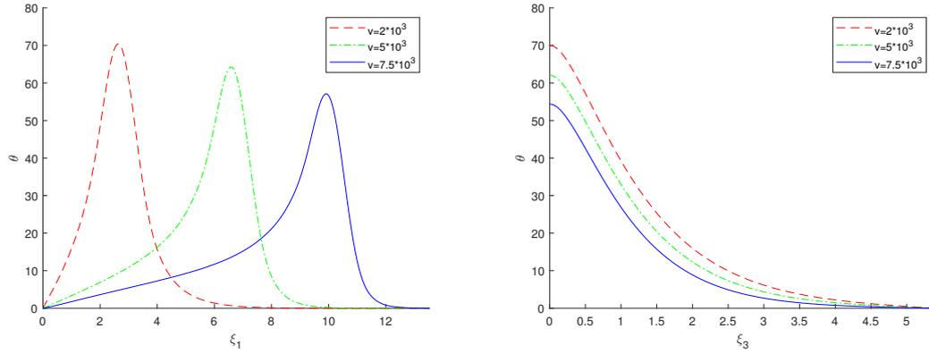
Figure 12: Top surface temperatures in the  $\xi_1$ -direction(left) and temperatures in the  $\xi_3$ -direction(right) of the medium subjected to a circular laser beam with different moving speeds under  $K_\tau = 1$ .
