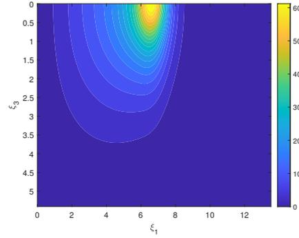
(c) The contour of the temperature in the  $\xi_3$ -direction when  $\xi_2 = W/2$ .
