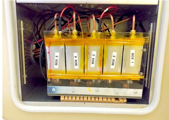
Figure 5: Photograph of the climate chamber (with door open) after being loaded with the boxes containing the tiles.
