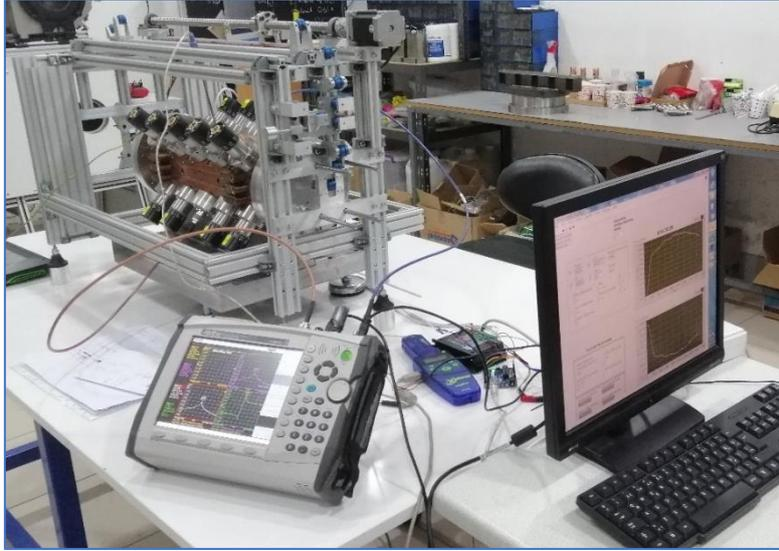
Figure 4: The experimental setup for the bead-pull measurements of the PTAK-RFQ module 0 at KAHVELab.
