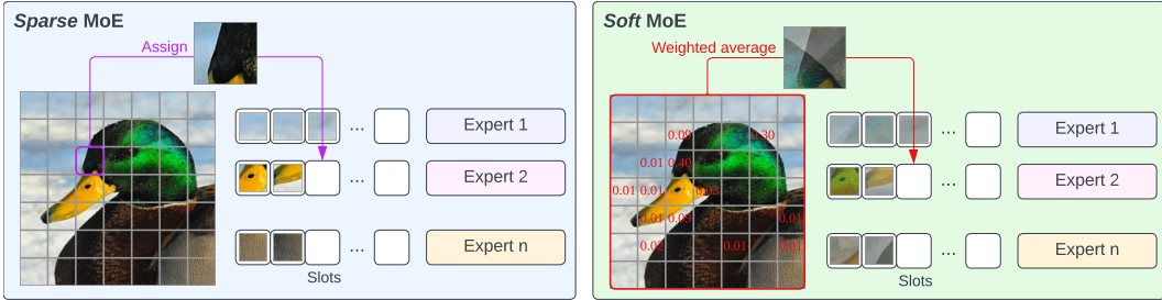
Figure 1: Sparse and Soft MoE layers. While the router in Sparse MoE layers (left) learns to assign individual input tokens to each of the available slots, in Soft MoE layers (right) each slot is the result of a (different) weighted average of all the input tokens. Learning to make discrete assignments introduces several optimization and implementation issues that Soft MoE sidesteps. Appendix G visualizes learned distributions of soft-assignments by Soft MoE.
