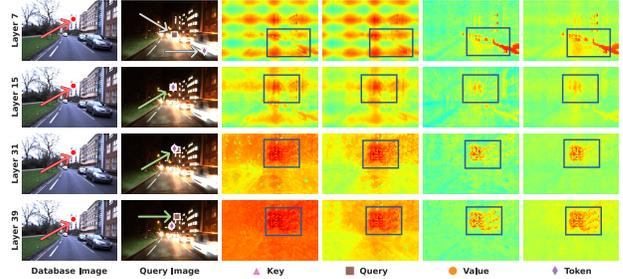
Fig. 3. Qualitative ablation comparing the absolute-scale similarity maps of features from different DINOv2 *layers* and *facets*. **Layer 31 value facet has the sharpest contrast** in the similarity map, which is **crucial for robustness against distractors within an image**.
