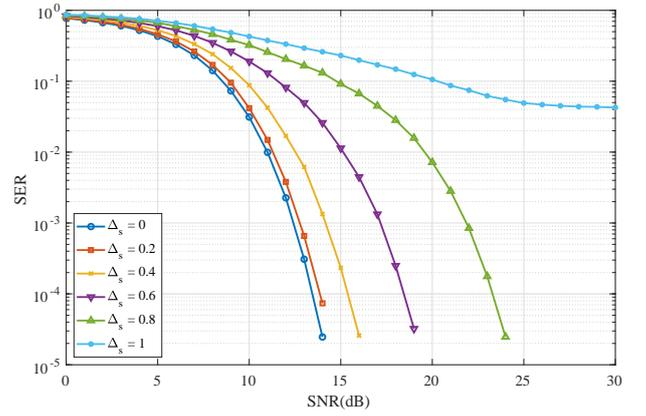
(b) SF = 4 and raised-cosine chip waveform
