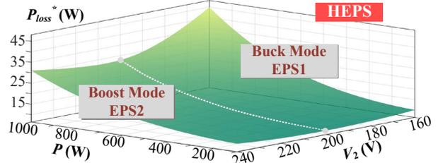
Fig. 16. Efficiency performance of the proposed AI-based HEPS modulation in the entire voltage and power ranges.
