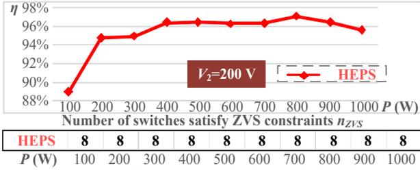
Fig. 31. Experimental efficiency ( $\eta$ ) and ZVS performance ( $n_{ZVS}$ ) of the proposed HEPS approach in unit gain mode when  $V_2 = 200$  V.
