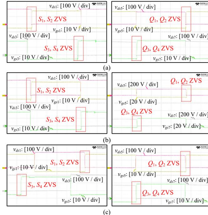
Fig. 24. ZVS waveforms  $v_{ds1}$ ,  $v_{gs1}$ ,  $v_{ds3}$ ,  $v_{gs3}$ ,  $v_{ds5}$ ,  $v_{gs5}$ ,  $v_{ds7}$ ,  $v_{gs7}$ , when  $V_2 = 160$  V and: (a)  $P = 1000$  W; (b)  $P = 500$  W; (c)  $P = 100$  W.
