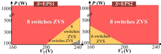
Fig. 14. ZVS ranges of EPS1 and EPS2 with the obtained optimal  $D_{in}$ .
