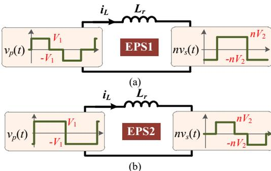
Fig. 4. Equivalent circuits of DAB converter under: (a) EPS1; (b) EPS2.
