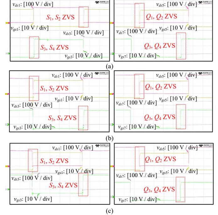
Fig. 25. ZVS waveforms  $v_{ds1}$ ,  $v_{gs1}$ ,  $v_{ds3}$ ,  $v_{gs3}$ ,  $v_{ds5}$ ,  $v_{gs5}$ ,  $v_{ds7}$ ,  $v_{gs7}$ , when  $V_2 = 240$  V and: (a)  $P = 1000$  W; (b)  $P = 500$  W; (c)  $P = 100$  W.
