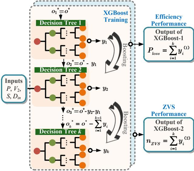
Fig. 9. Boosting training process of XGBoost.
