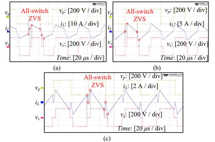
Fig. 22. Experimental waveforms under boost mode when  $V_2$  is 240 V and: (a)  $P = 1000$  W; (b)  $P = 500$  W; (c)  $P = 100$  W.
