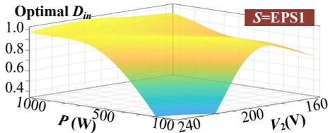
Fig. 12. Optimal  $D_{in}$  for strategy EPS1 as obtained by Stage II.
