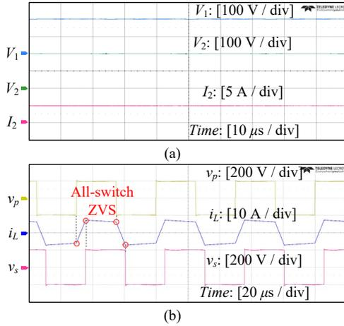
Fig. 19. Experimental waveforms under rated conditions when  $P$  is 1000 W and  $V_2$  is 200 V: (a)  $V_1$ ,  $V_2$  and  $I_2$ ; (b)  $v_p$ ,  $i_L$  and  $v_s$ .
