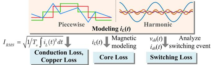
Fig. 7. Modeling efficiency.
