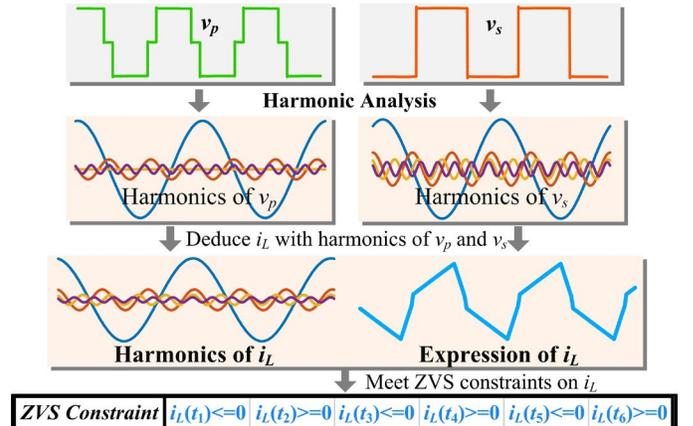
Fig. 6. Example of harmonic approach for modeling ZVS.
