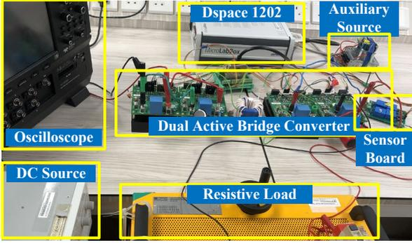
Fig. 18. Hardware platform for experimental validation.
