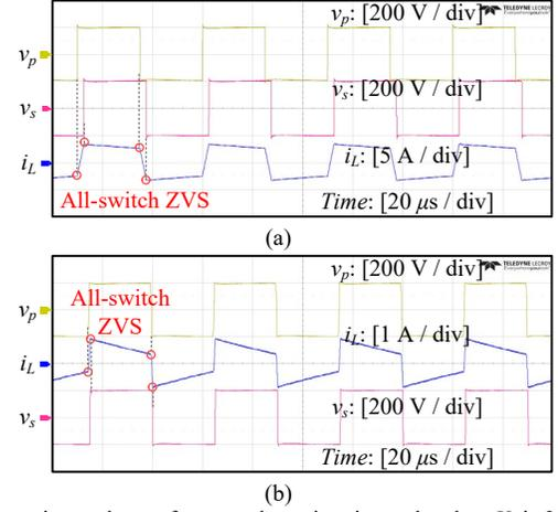
Fig. 20. Experimental waveforms under unit gain mode when  $V_2$  is 200 V and: (a)  $P = 500$  W; (b)  $P = 100$  W.
