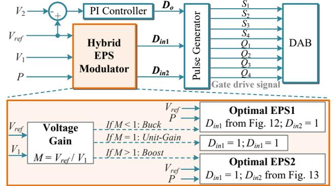
Fig. 17. Control diagram of the proposed AI-based HEPS modulation.
