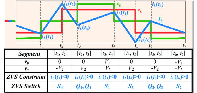
Fig. 5. Example of piecewise approach for modeling ZVS.
