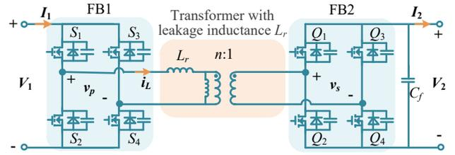
Fig. 1. Topology of a non-resonant DAB converter with leakage inductance  $L_r$ .
