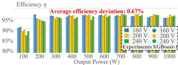
Fig. 32. Comparison between theoretical efficiency given by XGBoost-1 and experimental results.
