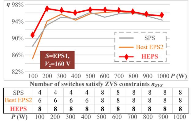
Fig. 29. Experimental efficiency ( $\eta$ ) and ZVS performance ( $n_{ZVS}$ ) of SPS, best EPS2, and the proposed HEPS approach in buck mode when  $V_2 = 160$  V.
