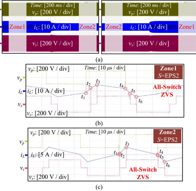
Fig. 27. Experimental waveforms during load steps when  $V_2 = 240$  V: (a)  $v_p$ ,  $i_L$  and  $v_s$  when  $P$  steps from 1000 W to 500 W and from 500W to 1000 W; (b) enlarged view of Zone1; (c) enlarged view of Zone2.
