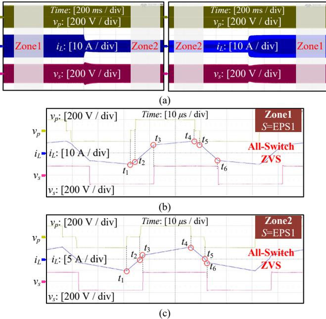
Fig. 28. Experimental waveforms during load steps when  $V_2 = 160$  V: (a)  $v_p$ ,  $i_L$  and  $v_s$  when  $P$  steps from 1000 W to 500 W and from 500W to 1000 W; (b) enlarged view of Zone1; (c) enlarged view of Zone2.
