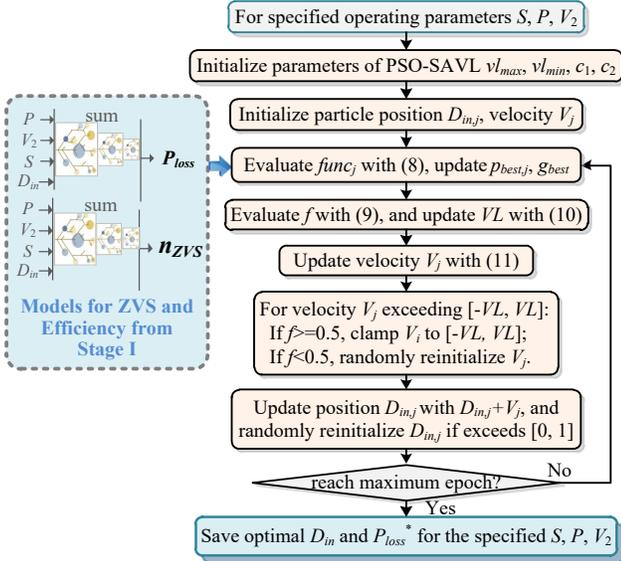
Fig. 11. Flowchart of PSO-SAVL applied in Stage II.
