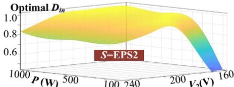
Fig. 13. Optimal  $D_{in}$  for strategy EPS2 as obtained by Stage II.
