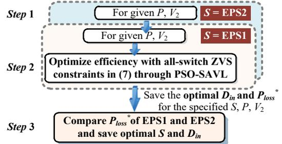
Fig. 10. Flowchart of Stage II of the proposed AI-based HEPS modulation.
