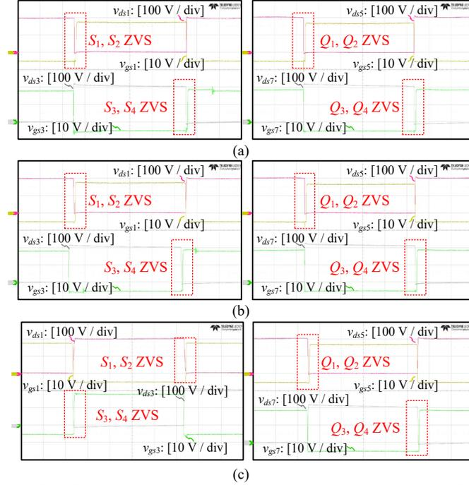
Fig. 23. ZVS waveforms  $v_{ds1}$ ,  $v_{gs1}$ ,  $v_{ds3}$ ,  $v_{gs3}$ ,  $v_{ds5}$ ,  $v_{gs5}$ ,  $v_{ds7}$ ,  $v_{gs7}$ , when  $V_2 = 200$  V and: (a)  $P = 1000$  W; (b)  $P = 500$  W; (c)  $P = 100$  W.
