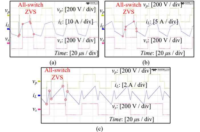
Fig. 21. Experimental waveforms under buck mode when  $V_2$  is 160 V and: (a)  $P = 1000$  W; (b)  $P = 500$  W; (c)  $P = 100$  W.
