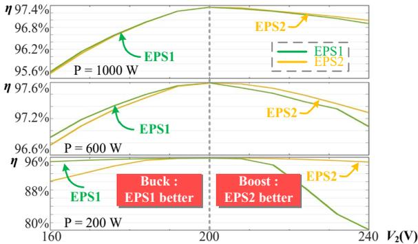
Fig. 15. Optimal efficiency of EPS1 and EPS2 with the obtained optimal  $D_{in}$ .
