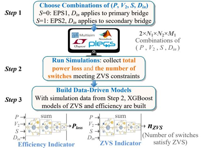
Fig. 8. Flowchart of Stage I of the proposed AI-based HEPS modulation.
