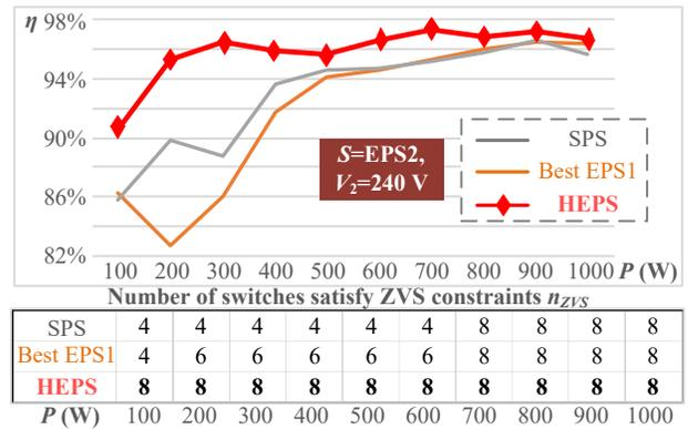
Fig. 30. Experimental efficiency ( $\eta$ ) and ZVS performance ( $n_{ZVS}$ ) of SPS, best EPS1, and the proposed HEPS approach in boost mode when  $V_2 = 240$  V.
