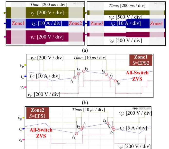
Fig. 26. Experimental waveforms during voltage steps when load resistance is  $57.6 \Omega$ : (a)  $v_p$ ,  $i_L$  and  $v_s$  when  $V_2$  steps from 240 V to 160 V and from 160 V to 240 V; (b) enlarged view of Zone1; (c) enlarged view of Zone2.
