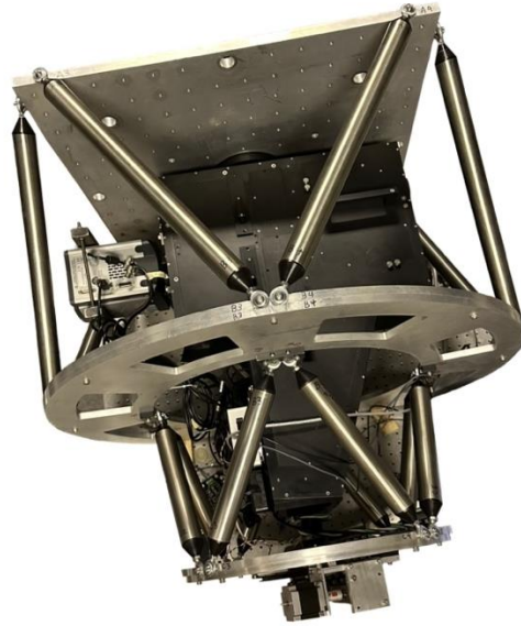
Figure 4: Left: A SolidWorks rendering of the RIPS housing in its rotating cage known as the ‘rotiserizer.’ Right: RIPS as built.
