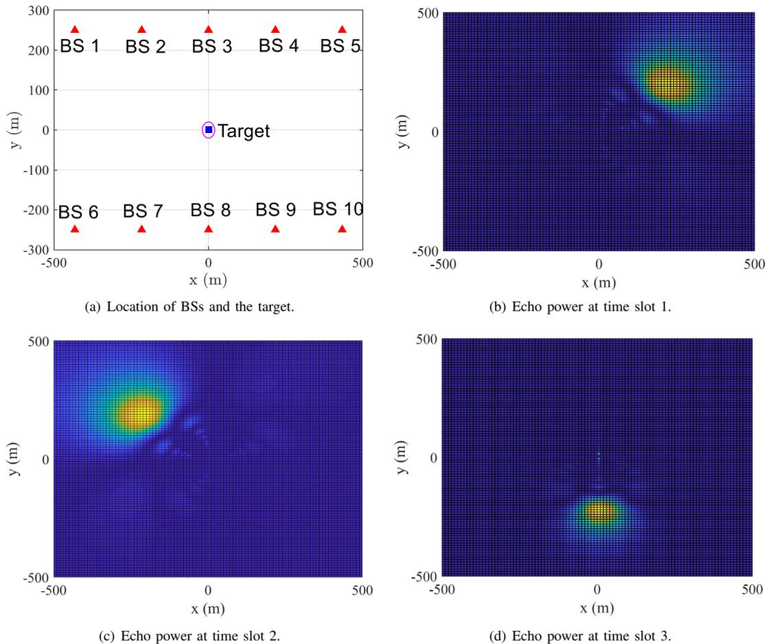
Fig. 3. Echo signals power at different locations.
