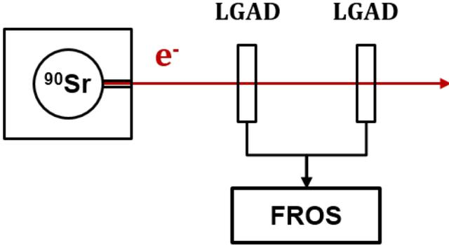
Fig. 5. Scheme of the function validation to the FROS. Two LGAD detectors are placed in line to measure the collimated electrons from the  $^{90}\text{Sr}$  source.
