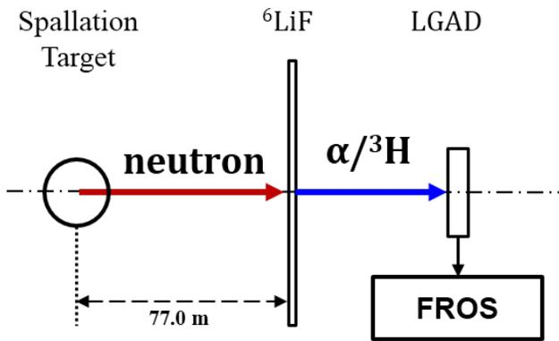
Fig. 3. Experimental scheme of the detector setup for  ${}^6\text{Li}(n, T)\alpha$ . (Not to scale)
