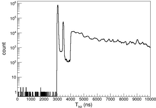
Fig. 7. Distribution of the arrival time of the signals referring to the  $T_0$  signal. The double peak in the left is the gamma flash produced in the spallation process. Two peaks are observed because the accelerator works in double bunch mode.
