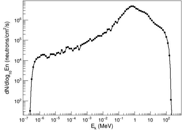
Fig. 1. Kinetic energy spectrum of the neutron provided by Back-n, spanning from thermal neutron energy to several hundreds of MeV. [13]
