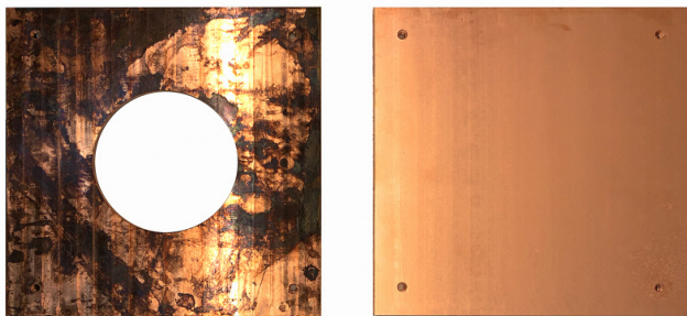
Fig. 14: Photos of NOSV copper samples before ( left ) and after ( right ) chemical surface cleaning.
