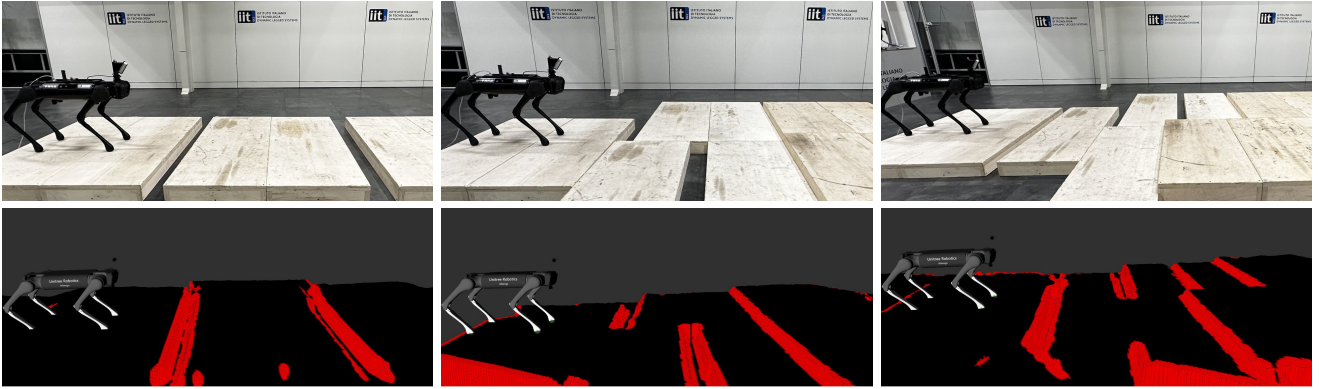
Fig. 4. The proposed test scenarios (top) with the related foot costmaps (bottom). Starting from the left, we show Scenario I, Scenario II, and Scenario III. Furthermore, in the foot costmaps the areas which are not considered safe are shown in red and the traversable areas are shown in black.
