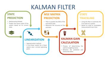
Fig. 5. A standard procedure based on the Kalman filter.
