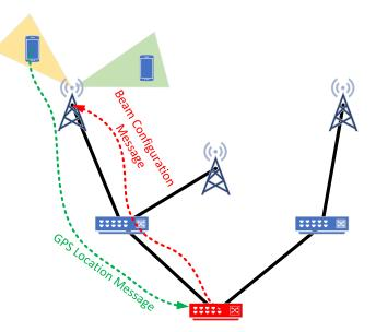
Fig. 6. Basic block diagram of Location-Assisted BF
