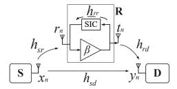
Fig. 1. Equivalent IIR channel model.
