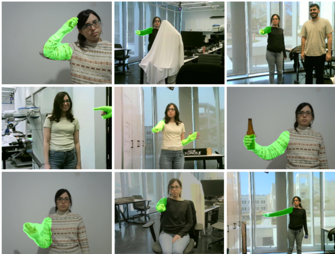
Fig. 10. Arm segmentation examples outputted by PointingNet-S in various scenarios of multiple participants, occlusions, dual-arm lift, sitting down and holding objects. The segmentation is performed for any lifted arm regardless of pointing or not. Classification later determines if pointing indeed occurs.
