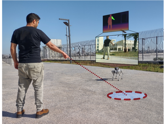
Fig. 1. A user directs a quadruped robot to a target position by pointing. The robot observes the user through an RGB camera. PointingNet identifies a pointing gesture and estimates its position and direction. Once the target has been calculated, the robot plans motion and moves to the target.
