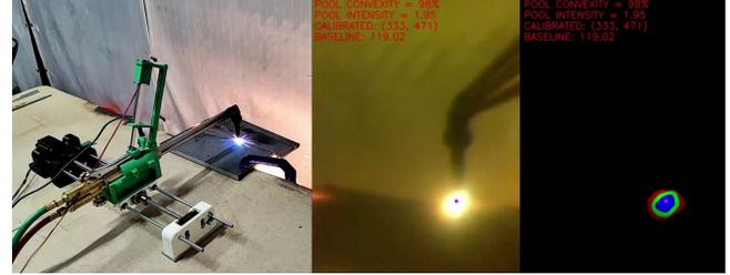
Fig. 1: The proposed vision-based control algorithm enables the 1-DOF cutting robot to autonomously cut steel plates of different thicknesses. **Left:** Third-person view of the robot during control. **Center:** Eye-in-hand view of the metal surface showing the heat pool. **Right:** Processed stream of the eye-in-hand footage focusing on the shown heat pool.
