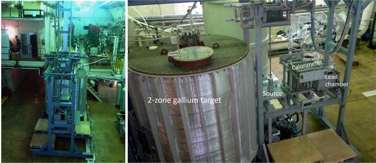
Figure 3.3: Left: A photograph of the Baksan Neutrino Observatory showing the BEST two-zone target in the foreground and the mixing reactors, with their red cap motor drives in the background. Right: A photograph of the two-zone target, the source, the calorimeter and the lead shield for  $\gamma$  spectrum measurements.
