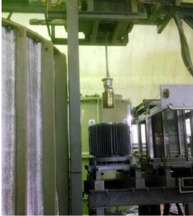
Figure 3.4: A photograph of the BEST source as it is being removed from its transport container. To the right side of the photo, the calorimeter can be seen.
