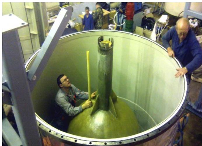
Figure 3.2: A photograph of the two-target volume during assembly.
