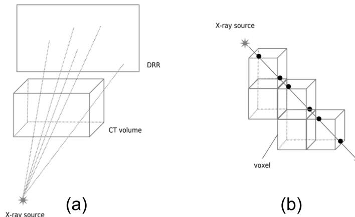
Figure 3: (a) X-rays passing through an object, resulting in a single projection on a plane. (b) targeted X-ray beam passing through a voxel.
