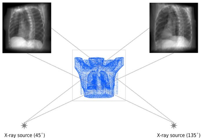
Figure 1: Dual X-ray setup. Two X-rays irradiate the patient, and their real-time fusion with CT scans enables precise patient positioning while accounting for potential misalignments. In this study, we adopt a similar strategy, setting our two ray source angles at  $45^\circ$  and  $135^\circ$ .
