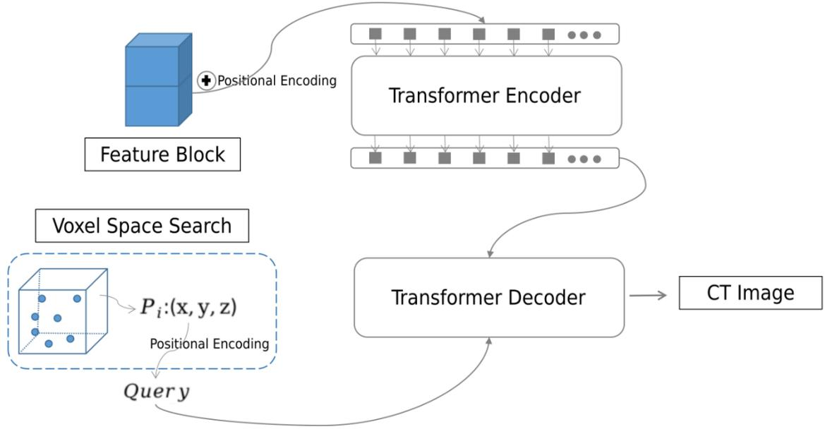
Figure 5: Structure of the transformer.
