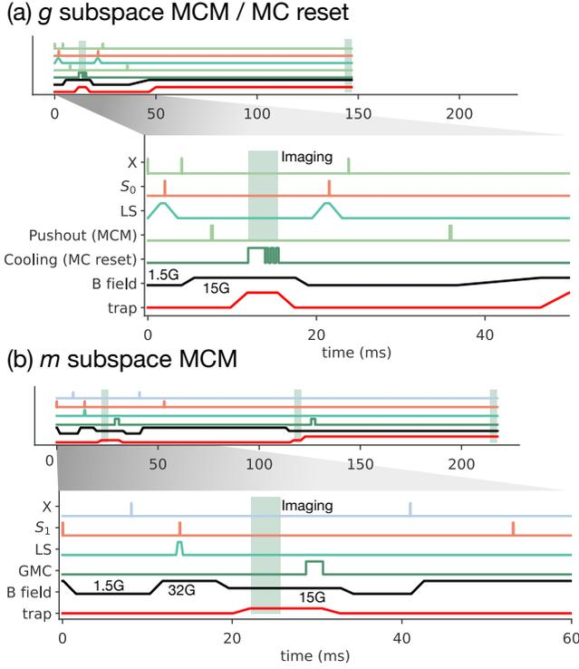
FIG. A6. Experimental sequence of the MCOs, with the timing is counted after the initial imaging and state preparation. For MCM, the green shaded region indicates imaging. (a) Sequence for the ground-state MCM and MC reset. Both share a similar experimental sequence, except for the spin detection, cooling and spin reset. (b) Sequence for the metastable MCM. Here, an extra image is taken at the end to assess atom loss.
