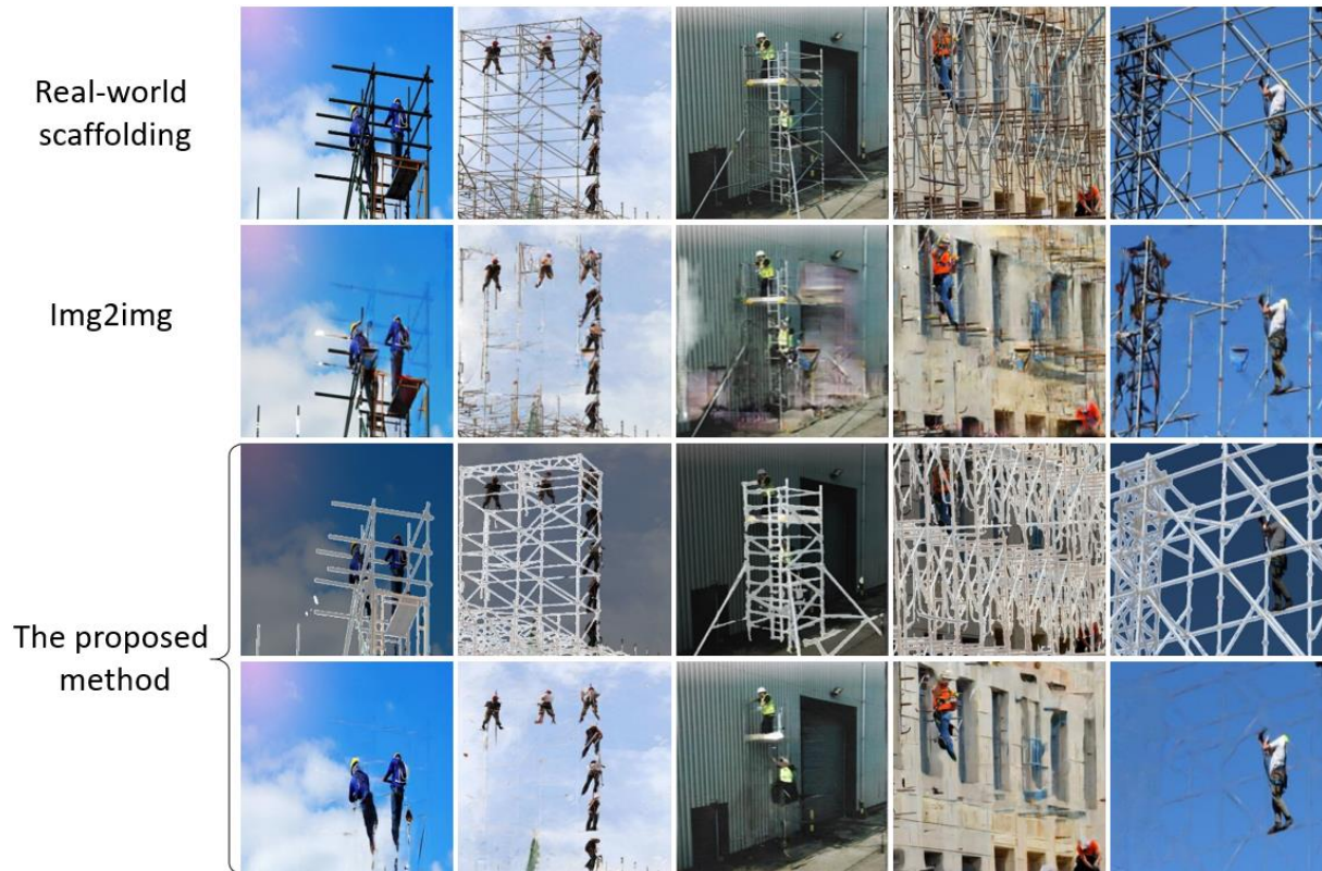
Figure 6. Real-world scaffold occlusion removal. The amplified details from left to right are cut from real-world scaffolding, results of the img2img method, and results of the proposed method.
