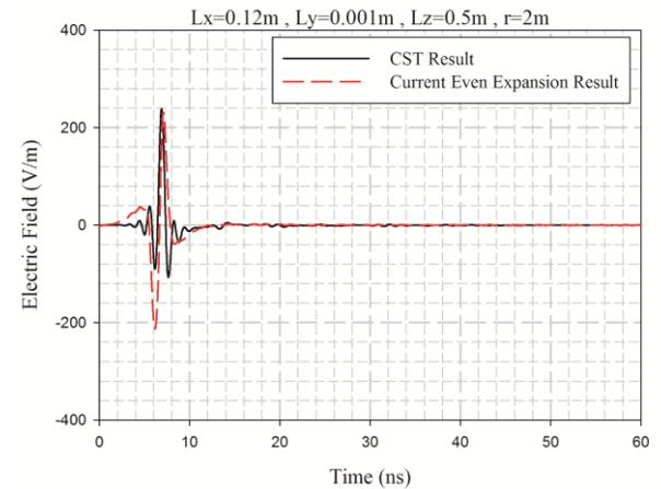
Fig. 11: The Far-field radiation calculated by the second method and CST results, for the slot with  $L_x=0.12m$ ,  $L_y=0.001m$ ,  $L_z=0.5m$ ,  $r=2m$ .
