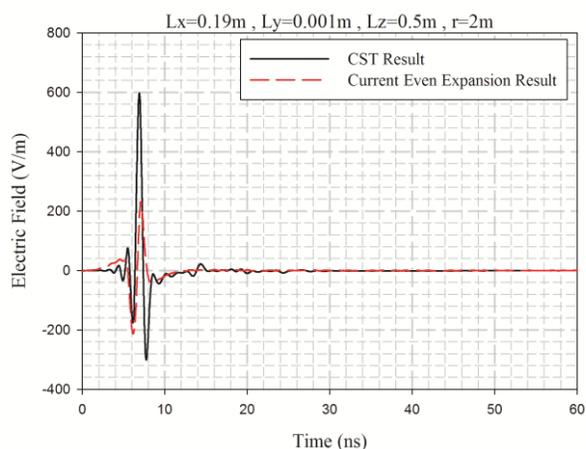
Fig. 12: The Far-field radiation calculated by the second method and CST results, for the slot with  $L_x=0.19\text{m}$ ,  $L_y=0.001\text{m}$ ,  $L_z=0.5\text{m}$   $r=2\text{m}$ .
