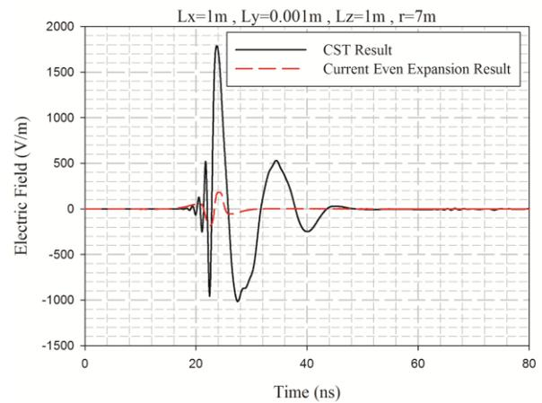
Fig. 10: The Far-field radiation calculated by the second method and CST results, for the slot with  $L_x=1m$ ,  $L_y=0.001m$ ,  $r=4m$ .
