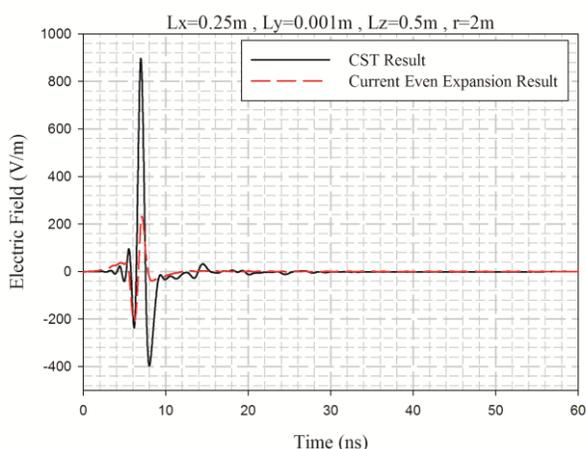
Fig. 13: The Far-field radiation calculated by the second method and CST results, for the slot with  $L_x=0.25\text{m}$ ,  $L_y=0.001\text{m}$ ,  $L_z=0.5\text{m}$   $r=2\text{m}$ .
