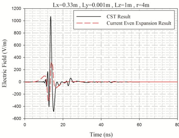
Fig. 8: The Far-field radiation calculated by the second method and CST results, for the slot with  $L_x=0.33m$ ,  $L_y=0.001m$ ,  $r=4m$ .
