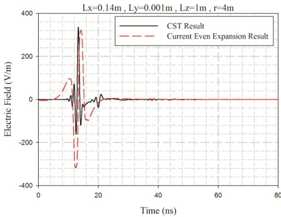
Fig. 7: The Far-field radiation calculated by the second method and CST results, for the slot with  $L_x=0.14m$ ,  $L_y=0.001m$ ,  $r=4m$ .
