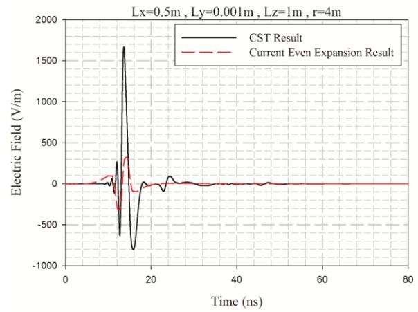
Fig. 9: The Far-field radiation calculated by the second method and CST results, for the slot with  $L_x=0.5m$ ,  $L_y=0.001m$ ,  $r=4m$ .
