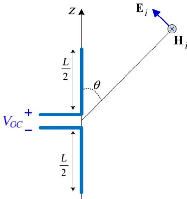
Fig. 5: A linear antenna in receiving mode.
