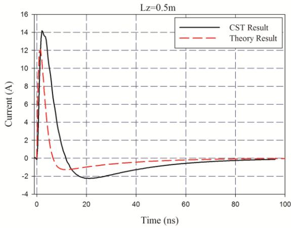
Fig. 6: The Induced current in the resistance, calculated by theory and simulation.
