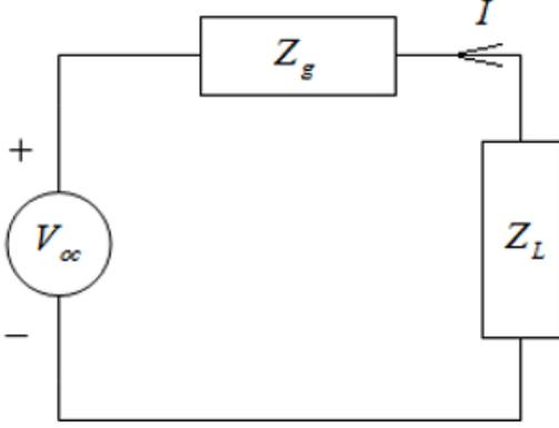
Fig. 4: The equivalent circuit of an antenna in receiving mode.
