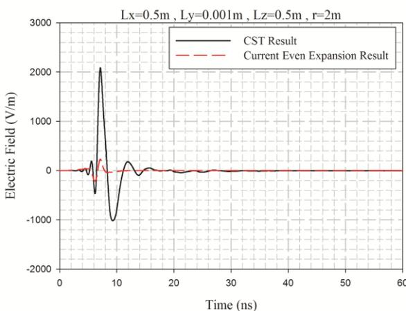
Fig. 14: The Far-field radiation calculated by the second method and CST results, for the slot with  $L_x=0.5\text{m}$ ,  $L_y=0.001\text{m}$ ,  $L_z=0.5\text{m}$   $r=2\text{m}$ .
