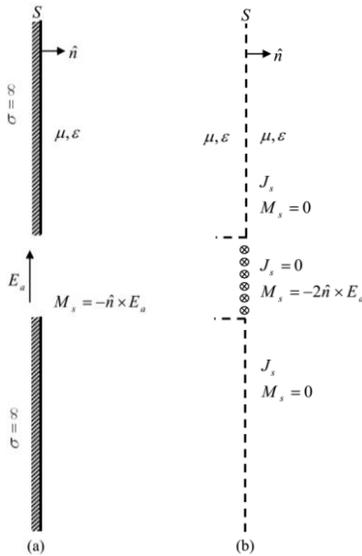
Fig. 2: Equivalent model for an aperture in the planar conducting screen of infinite extent.
