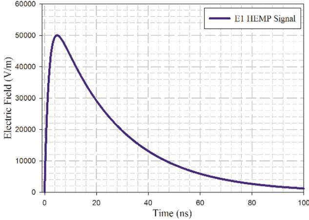
Fig. 1: The E1 HEMP waveform.
