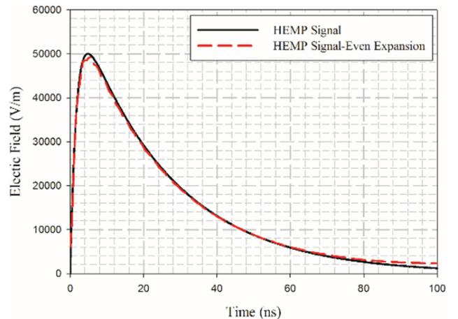
Fig. 3: The HEMP signal and its Fourier's even expansion.
