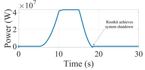
Fig. 9. Power magnitude as measured at the PMM during a system shutdown caused by the rootkit attack.
