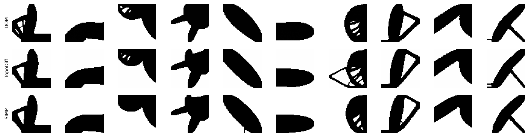
Figure 13: Comparison DOM and TopoDiff-GUIDED generation with 100 steps.
