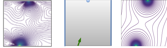
Figure 5: Comparison of iterative (left), sparse (center), and dense single-step (right) conditioning fields for a Constrained Diffusion Model. Unlike the expensive iterative FEA method, the physics-inspired fields offer a cost-effective, single-step approximation that’s domain-agnostic and scalable.
