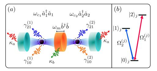
FIG. 1. (a) Schematic diagram of a cavity-atom-mechanics system. (b) Two lasers with intensities  $\propto$  to  $\Omega_1^{(j)}$  and  $\Omega_2^{(j)}$  driving the three-level *j*-atom, which are resonant with the transitions of the levels  $|2\rangle_j \longleftrightarrow |0\rangle_j$  and  $|1\rangle_j \longleftrightarrow |0\rangle_j$ , respectively.
