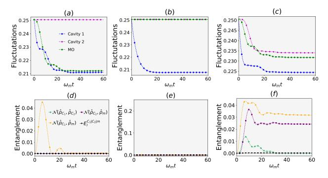
FIG. 6. Dissipative time evolution of QF (top panel) and entanglement (bottom panel) of the bosonic modes when the squeezing is induced in the first cavity. Managing the Jaynes-Cummings couplings so that the tripartite couplings are:  $(a, d) \Lambda_1 = 1$ ,  $\Lambda_2 = 0$ ;  $(b, e) \Lambda_1 = 0$ ,  $\Lambda_2 = 1$ ;  $(c, f) \Lambda_1 = 1, \Lambda_2 = 1.1$ . Other parameters are the same as in Fig.5. Additionally with  $\phi_{c_1} = \phi_{c_2} = \pi/4$ ,  $\phi_m = -\pi/4$ .
