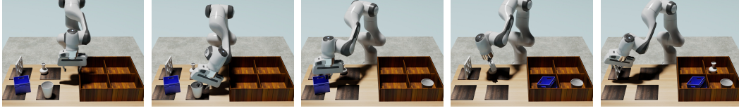
Figure 1: Long-horizon task visualization. We visualize the initial state and each intermediate pick state for the pick-and-place task. Note there is significant variation in geometry across each object, requiring the agent to perform a diverse series of grasps to complete the task.
