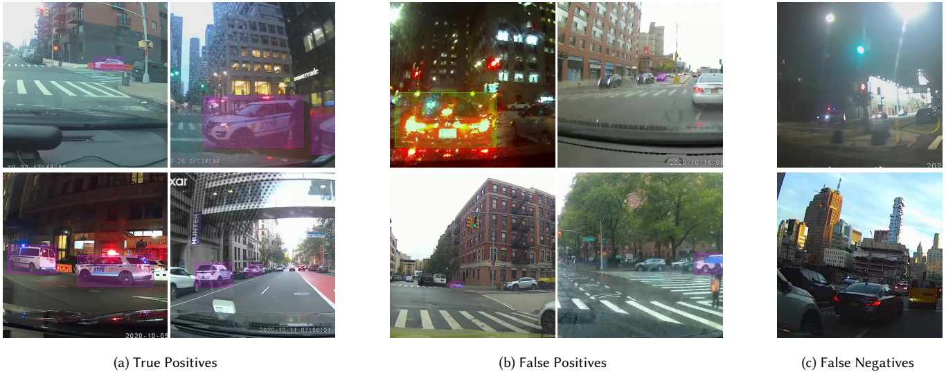
Fig. 3. Examples of police vehicle detections. Notice the different times of day, differing camera perspectives, and multiple types of vehicles. Initially, the object detection model was easily confused by NYC taxis, buses, white sedans, and white SUVs. As more training data was added, the model was more difficult to confuse, with incorrect classifications occurring typically with optical illusions and poor light conditions. Note that images are cropped and zoomed to better depict annotated regions; raw images are 1280x720.
