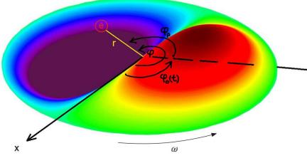
FIG. 2.  $E_z^{hf}$  component of rotating  $TM_{110}$  mode and the angles used to describe the electron rotation. Here,  $\varphi$  represents the angular position of the electron,  $\varphi_0(t)$  defines a rotating axis where  $E_z^{hf}$  has its maximum value, and  $\varphi_p(t)$  is the relative angular position of the electron.
