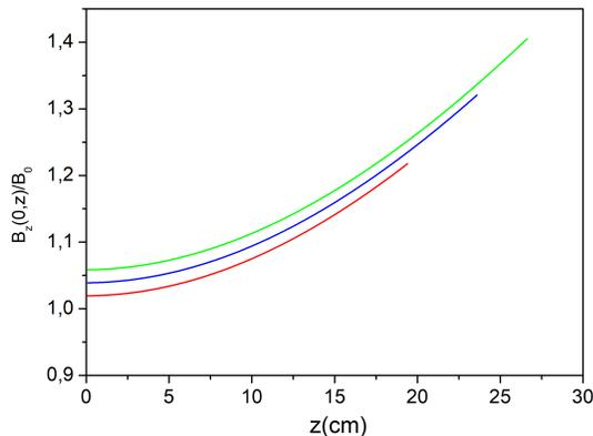
FIG. 12. Magnetic field profile to obtain exact resonance predicted by the model described in the present work for the injection energies of (i) 10 keV, (ii) 20 keV, and (iii) 30 keV.
