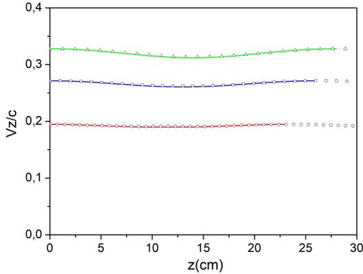
FIG. 6. Electron longitudinal velocity as a function of the  $z$  coordinate for the injection energies of (i)  $10\text{ keV}$ , (ii)  $20\text{ keV}$ , and (iii)  $30\text{ keV}$ , for the case of the uniform magnetostatic field of  $0.286\text{ T}$ . The solid lines correspond to the results obtained from the model described in the present work, and the circles, squares and triangles correspond to those obtained from the numerical solution of Eq.(2) by using the Boris method.
