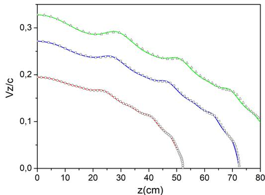
FIG. 10. Electron longitudinal velocity as a function of the  $z$  coordinate for the injection energies of (i) 10 keV, (ii) 20 keV, and (iii) 30 keV, for the case of linear magnetostatic field. The solid lines correspond to the results obtained from the model described in the present work, and the circles, squares, and triangles correspond to those obtained from the numerical solution of Eq.(2) by using the Boris method.
