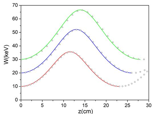
FIG. 4. Electron energy as a function of the  $z$  coordinate for the injection energies of (i) 10 keV, (ii) 20 keV, and (iii) 30 keV, for the case of the uniform magnetostatic field of 0.286 T. The solid lines correspond to the results obtained from the model described in the present work, and the circles, squares and triangles correspond to those obtained from the numerical solution of Eq.(2) by using the Boris method.
