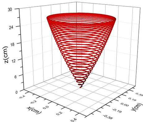
FIG. 16. The trajectory of an electron injected along the cavity axis with the energy of 30 keV for the case of exact resonance.
