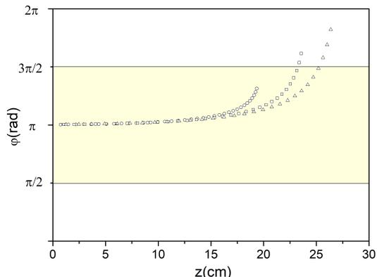
FIG. 13. Relative angular position of the electron as a function of the  $z$  coordinate for the injection energies of (i) 10 keV (circles), (ii) 20 keV (squares), and (iii) 30 keV (triangles), obtained from the numerical solution of Eq.(2) by using the Boris method.
