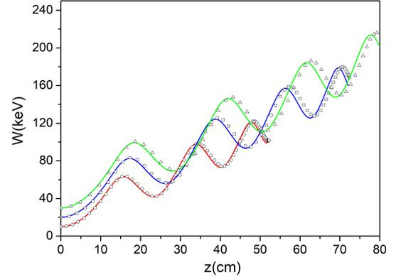
FIG. 8. Electron energy as a function of the  $z$  coordinate for the injection energies of (i)  $10\text{ keV}$ , (ii)  $20\text{ keV}$ , and (iii)  $30\text{ keV}$ , for the case of linear magnetostatic field. The solid lines correspond to the results obtained from the model described in the present work, and the circles, squares, and triangles correspond to those obtained from the numerical solution of Eq.(2) by using the Boris method.
