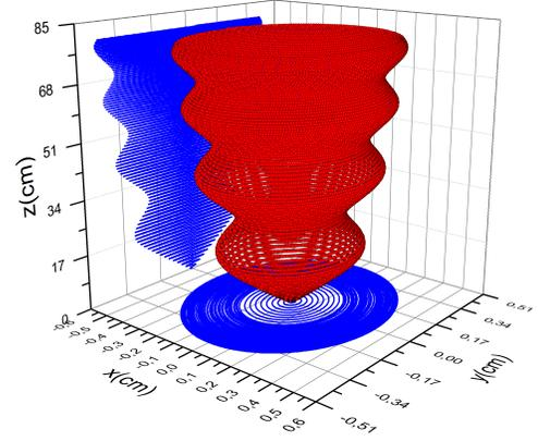
FIG. 7. The trajectory of an electron injected along the cavity axis with the energy of  $30\text{ keV}$  for the case of the linear magnetic field.
