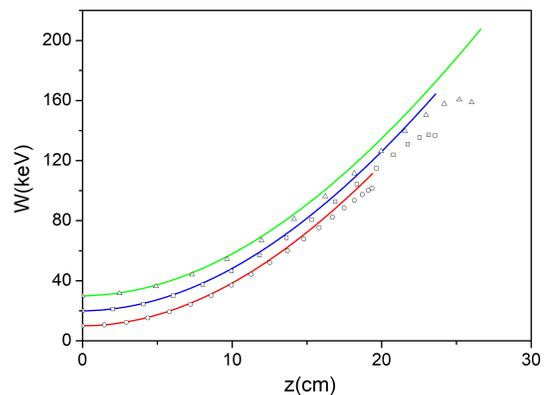
FIG. 11. Electron energy as a function of the  $z$  coordinate for the injection energies of (i) 10 keV, (ii) 20 keV, and (iii) 30 keV, for the case of exact resonance. The solid lines correspond to the results obtained from the model described in the present work, and the circles, squares, and triangles correspond to those obtained from the Boris method.
