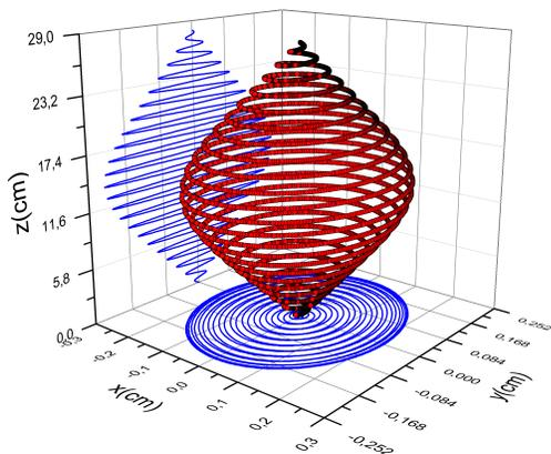
FIG. 3. The trajectory of an electron injected along the cavity axis with the energy of 30 keV for the case of the uniform magnetic field, and its projections onto the planes  $xy$  and  $yz$ .
