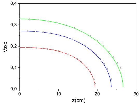
FIG. 14. Electron longitudinal velocity as a function of the  $z$  coordinate for the injection energies of (i) 10 keV, (ii) 20 keV, and (iii) 30 keV, for the case of exact resonance. The solid lines correspond to the results obtained from the model described in the present work, and the circles, squares and triangles correspond to those obtained from the numerical solution of Eq.(2) by using the Boris method.
