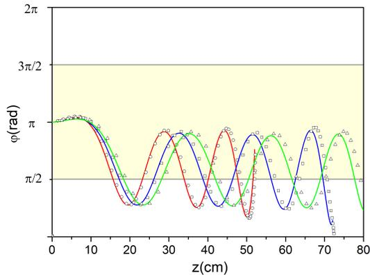
FIG. 9. Relative angular position of the electron as a function of the  $z$  coordinate for the injection energies of (i) 10 keV, (ii) 20 keV, and (iii) 30 keV, for the case of the linear magnetostatic field. The solid lines correspond to the results obtained from the model described in the present work, and the circles, squares, and triangles correspond to those obtained from the numerical solution of Eq.(2) by using the Boris method.
