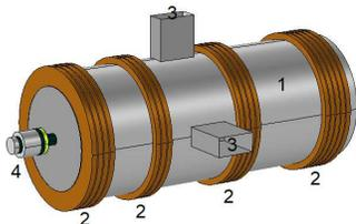
FIG. 1. Physical model scheme: 1-cavity, 2-magnetic coils, 3-microwave ports, 4-electron gun.
