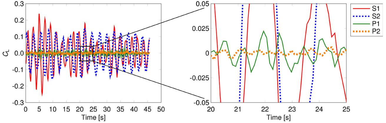
Extended Data Figure 9: Lift coefficient  $C_L$ . Left, time trace at statistical steady state of the lift coefficient  $C_L$  for the different models (see key at right) of *E. aspergillum* at  $Re = 2,000$ . The range of the oscillations in the porous models is two orders of magnitude less than that of the plain cylinder S1. Right, magnified view of boxed region.
