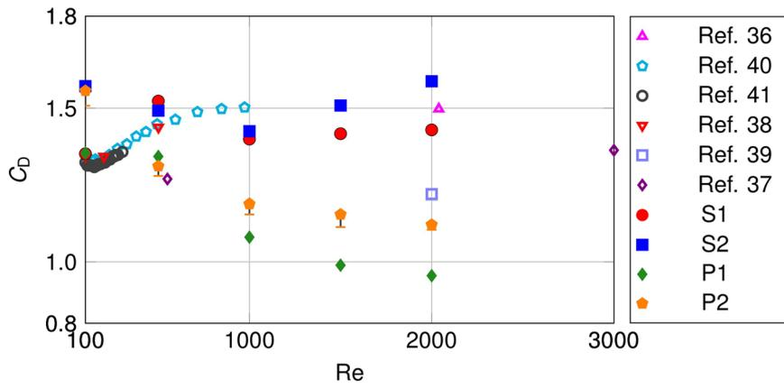
Extended Data Figure 6: Details of the drag coefficient. Zoomed-out view of main text Fig. 3c, with error bars identifying the range of predicted values of the drag coefficient  $C_D$  due to random morphological manipulations. These variations lead to a modest decrease, from 2.5% to 3.5% in the drag coefficient with respect to the pristine model.
