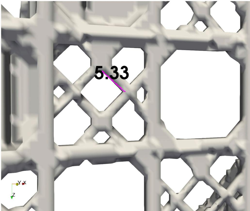
Extended Data Figure 1: Detail of the grid resolution. The grid resolution within the small fenestrae of *E. aspergillum* models is 5.33 lattice spacings.
