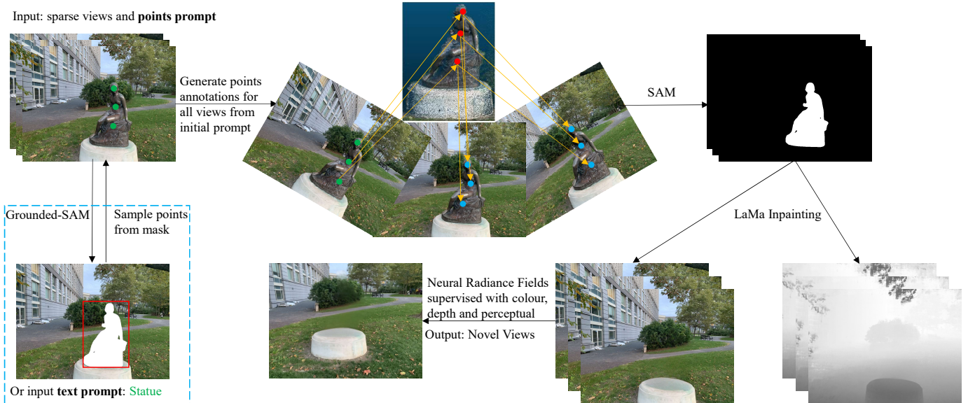
Fig. 1. An overview of our OR-NeRF’s framework. We start with sparse images and either points or text prompts. If a text prompt is used, we convert it into a points prompt by sampling points from the initial mask estimated using Grounded-SAM (Sec IV-A2). Next, we propagate the points annotations to all views by projecting them from 2D to 3D point cloud and back to 2D (Sec IV-A1). We utilize SAM to predict masks using these point annotations. LaMa is used to obtain color and depth priors. Finally, the scene after removal is reconstructed using Neural Radiance Fields supervised by color (Eq (3)), depth (Eq (5)), and perceptual (Eq (6)) cues simultaneously (Sec IV-B).
