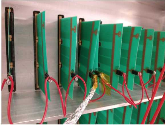
Figure 7: Shorting cards are used to group pads from three connectors at the back of the OROC into a single channel. The fourth card from the left is passivated on the lower two legs and connects with the upper leg only to the top connector. These 21 pads are opposite to the ^{55}\text{Fe} source and read out as the signal channel. The following card connects to the middle and lower connector in this row and the corresponding pad groups are connected to ground, as are all other pad groups which are not read out.
