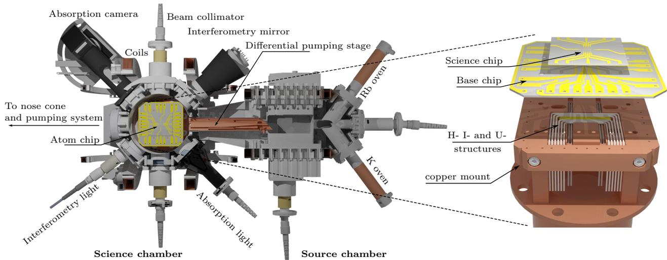
**Fig. 2** Model of the experimental chamber (left) divided into science- and source chamber. Detailed view of the three-layer atom chip (right)
