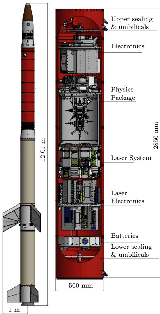
**Fig. 1** The scientific payload (in red) on top of the two engines of a VSB-30 sounding rocket (left) and detailed view of the experimental payload (right). The payload hull is separated into seven RADAX segments. Image from Elsen (2023).
