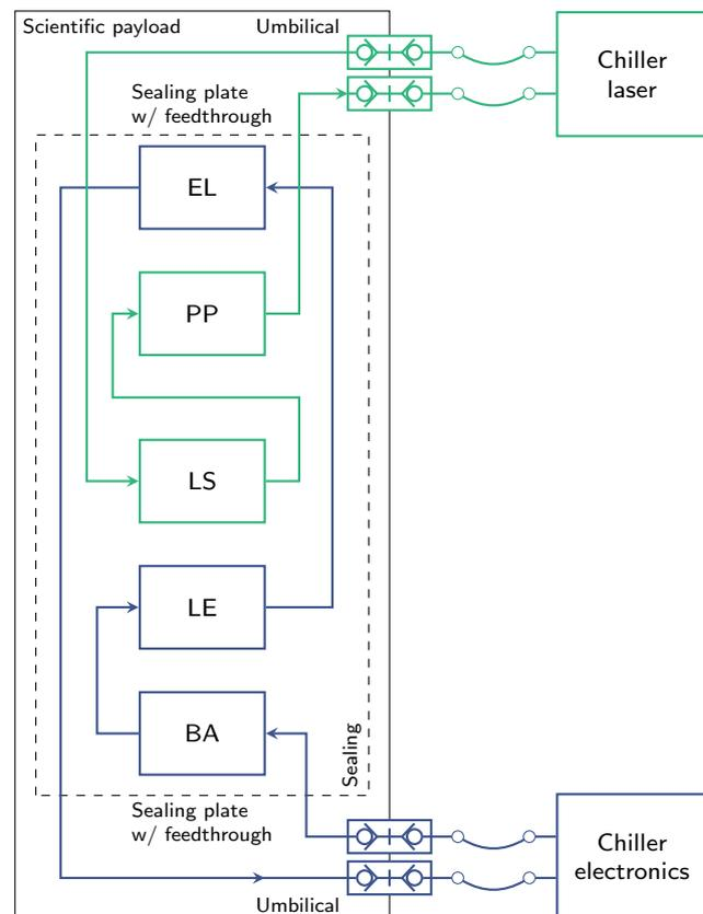
**Fig. 4** Schematic overview of the two cycle cooling concept within the TCS. The electronics cycle (in blue) feeds the subsystems BA, LE and EL and the laser cycle (in green) the LS and PP. Figure adapted from Elsen (2023).
