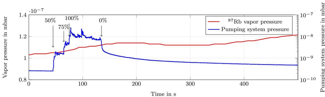
**Fig. 7** Vacuum pressure in PP pumping system (blue curve) and  $^{87}\text{Rb}$  vapour pressure in the source chamber (red curve) prior, during and after vibrational test of the longitudinal axis. The rms-value of vibration loads is increased to the final value in three steps, as indicated by the arrows. Figure adapted from Piest (2021).
