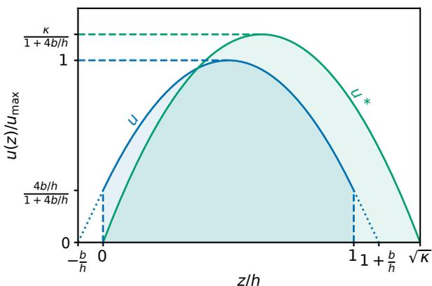
FIG. 1. Wall slip leads to an effective gap height  $h_{\text{eff}} = h\sqrt{\kappa}$ . The parameter  $\kappa$  is found by equating the  $z$ -average of the original velocity profile  $u(z)$  with that of  $u^*(z)$ , which is  $u$  shifted to yield zero slip.
