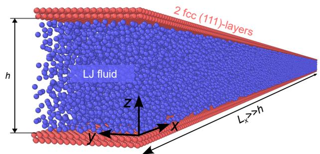
FIG. 4. Simulation setup for molecular dynamics simulations of confined fluids. One lateral dimension is much larger than the gap height.
