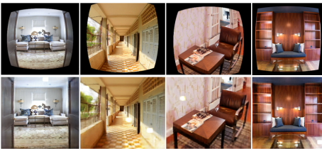
Fig. 3. The quick rectification performed by our WGAN enhanced Pix2Pix GAN model. 1 st row : original synthesized fisheye images; 2 nd Row : rectified images
