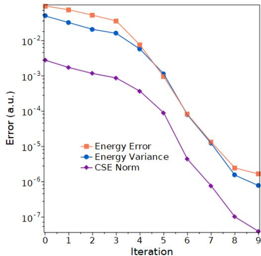
FIG. 1. Superlinear convergence of the energy error, variance, and least-squares CSE norm is shown for the fifth excited state of linear  $H_4$ .
