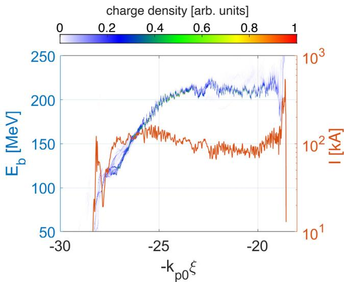
FIG. 6: Generation of electron beams with  $\sim 100$  kA current by sending a 1.2 PW laser pulse into a plasma with  $10^{19}$   $\text{cm}^{-3}$  density: the longitudinal phase space and the current profile at  $\omega_{p0}t = 400$ .
