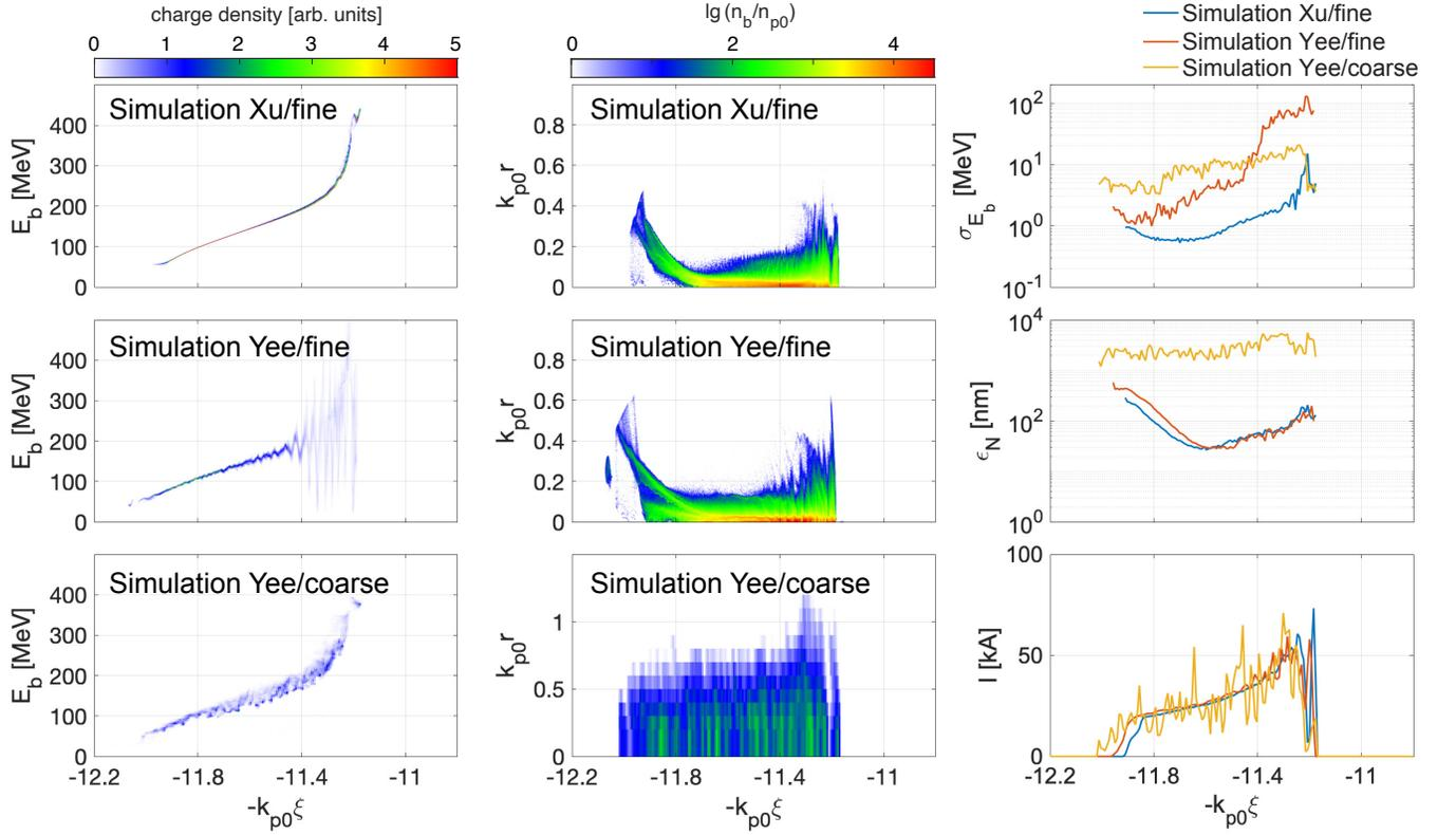
FIG. 8: Comparison of the injected beams at  $\omega_{p0}t = 250$  in a uniform plasma from simulations with different resolutions and different solvers. Simulation Xu/fine:  $dz = dr = \frac{1}{512}k_{p0}^{-1}$  and the Xu solver; Simulation Yee/fine:  $dz = dr = \frac{1}{512}k_{p0}^{-1}$  and the Yee solver; Simulation Yee/coarse:  $dz = \frac{1}{150}k_{p0}^{-1}$ ,  $dr = \frac{1}{10}k_{p0}^{-1}$  and the Yee solver.
