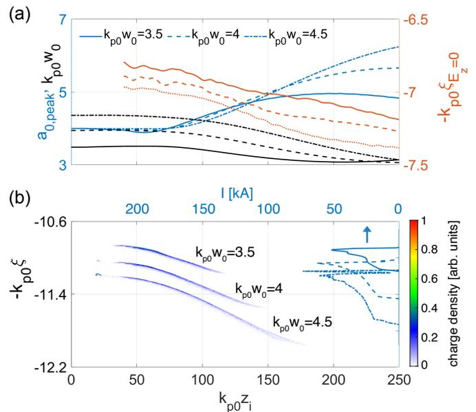
FIG. 4: (a) The evolution of the laser pulse driver and the plasma wake wave under different laser spot sizes:  $k_{p0}w_0 = 3.5, 4$  and  $4.5$ . (b) The charge density distribution of the injected electrons and their current profiles for these cases.
