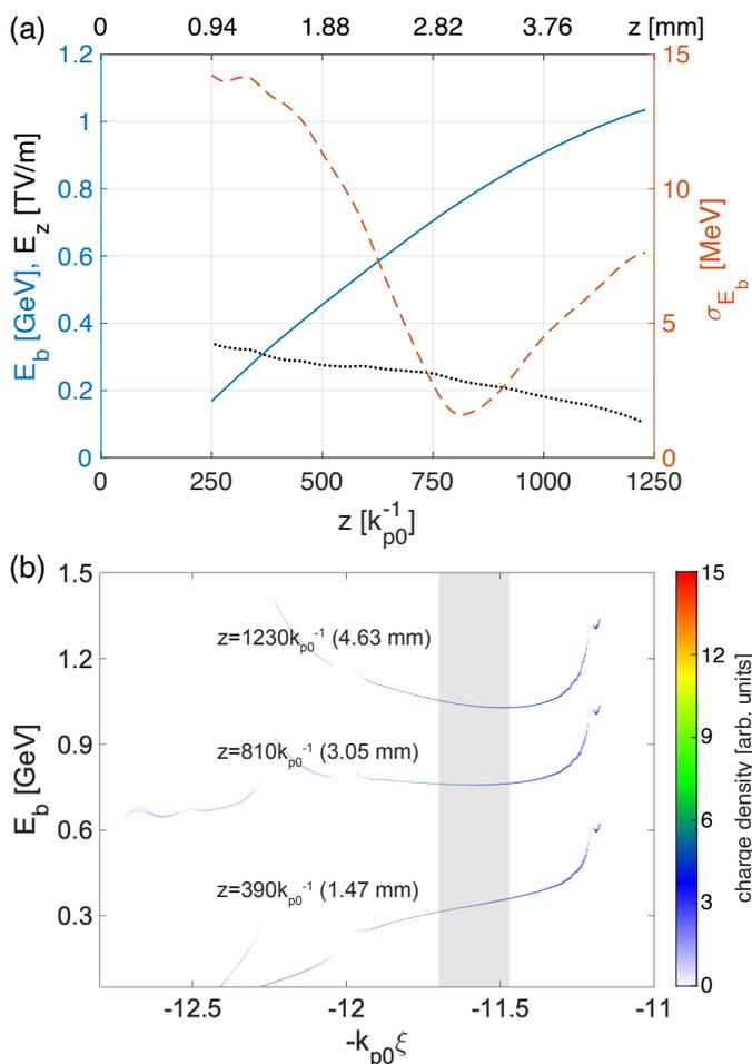
FIG. 3: (a) The evolution of the average energy (blue solid line) and the projected energy spread (red dashed line) of the core of the beam ( $g = 0$ ) and the acceleration gradient (black dotted line). (b) Longitudinal phase space of the injected electrons at three acceleration distances. The shadowed region represents the beam core.
