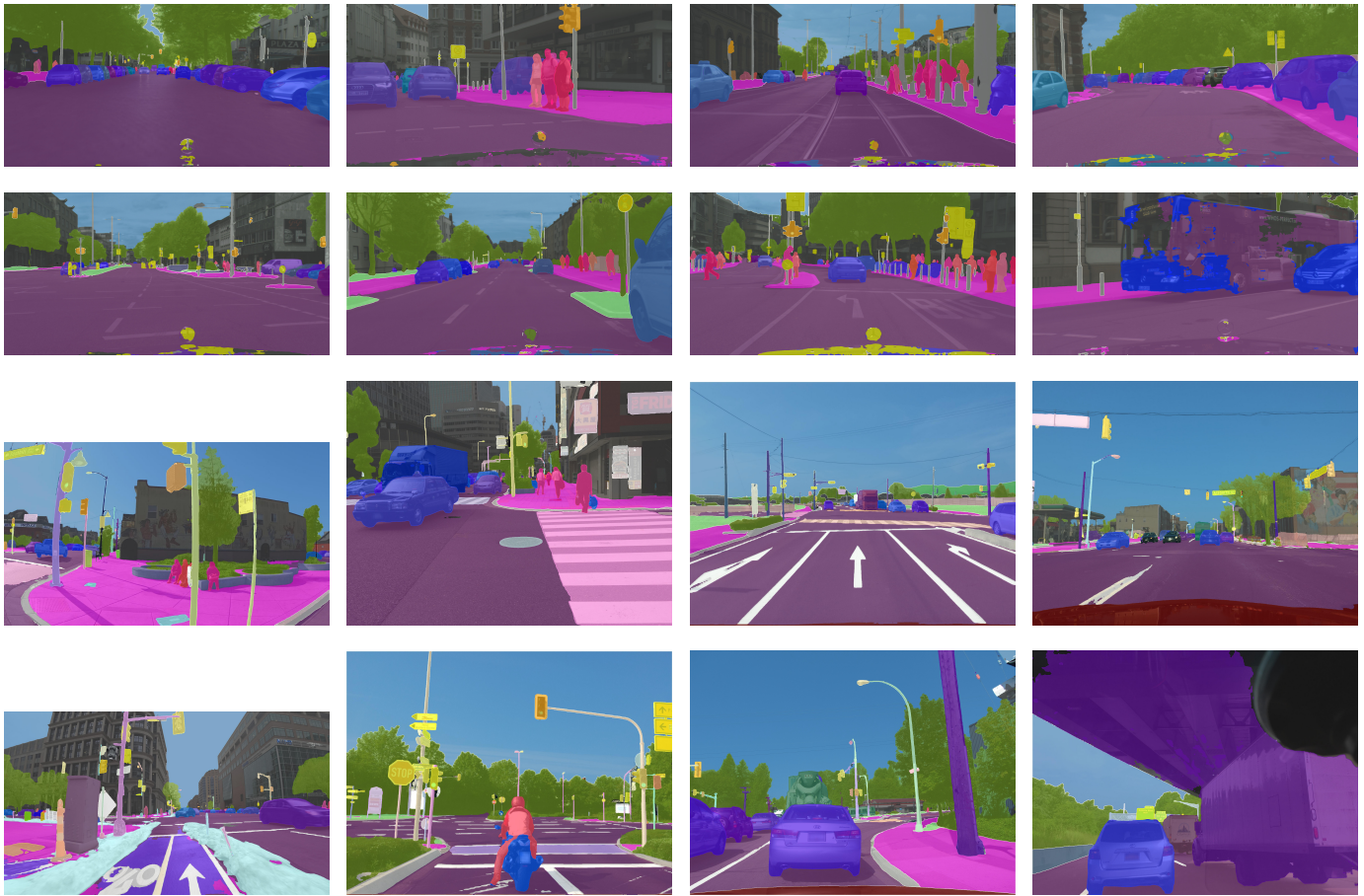
Fig. 4. Qualitative results on unseen images from the Cityscapes dataset [6] (first two rows) and the Mapillary Vistas dataset [23] (last two rows). Each mask prediction gets a unique color. The last column shows misclassifications, where RT-K-Net has problems finding all objects or predicting an accurate mask for rare classes.
