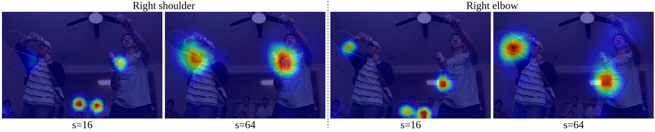
Figure 8. Visualization of visibility maps with different scales. A lower scale factor s indicate higher resolution in visibility maps.
