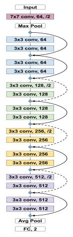
Fig. 5: Resnet18/Teacher architecture. The coloured blocks represent the convolution layers and the respective kernel sizes, output filters and the reduction of input size. The lines between the convolution layers represent residual connections, whereas the dashed represents that the input of the residual goes through a convolution for dimension consistency. The final FC layer is a dense layer.
