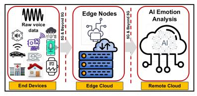
Fig. 1: State-of-the-art non-speech emotion-sensing system that transmits raw speech signals over the communication network for emotion analysis.
