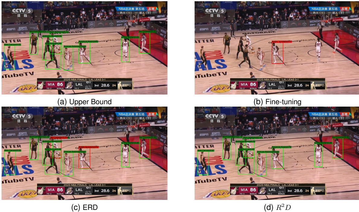
Fig. 5. Visualization of experimental results on NBA-IOD benchmark under the three-step setting: (a) Detection results with GFL training on all data; (b) Detection results with GFL by directly fine-tuning (Catastrophic Forgetting); (c) Incremental results of ERD; (d) Incremental results of R^2D .
