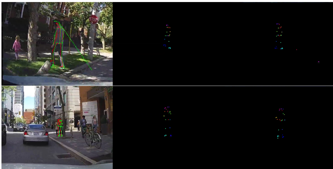
Figure 12: Example PIE@0.1 rendering results. From left: fragment of a source video with original pose data (red) and model output (green), normalized input pose data as dots, model output as dots.
