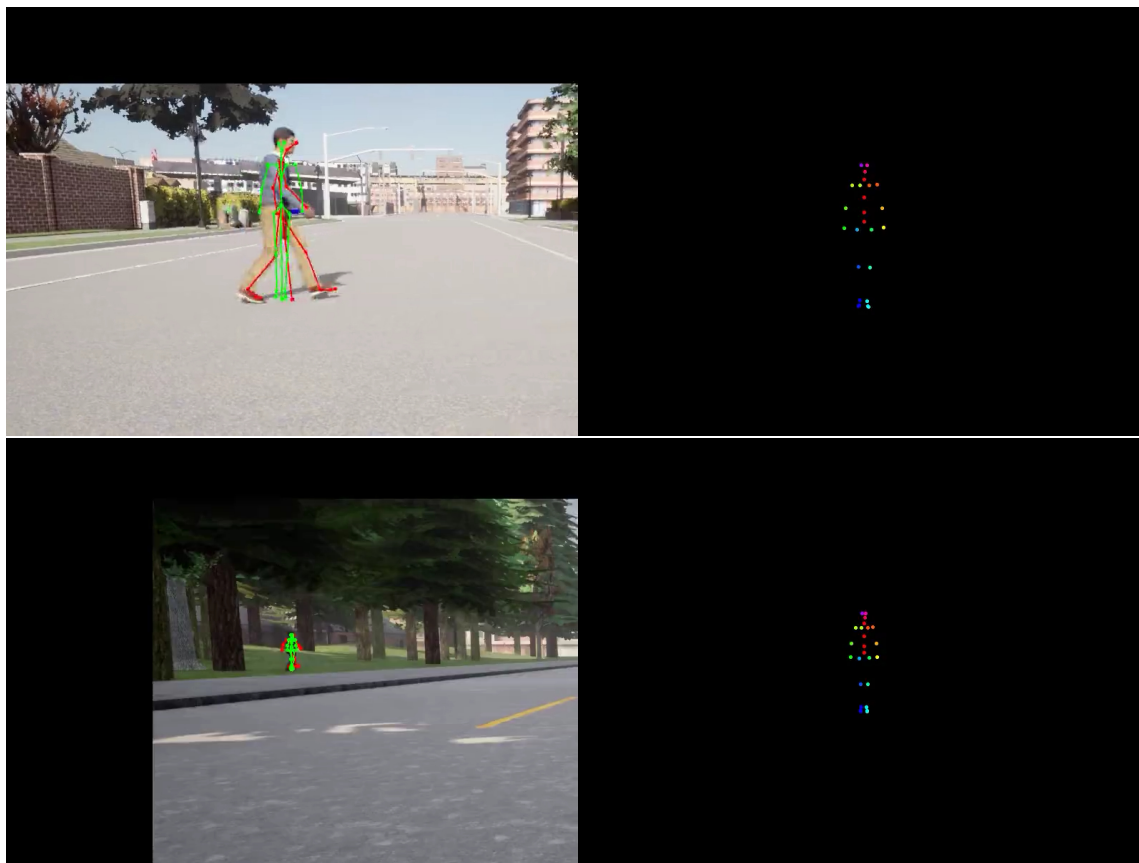
Figure 15: Visualization of pose estimation results. It can be seen that the model learned the average skeleton.
