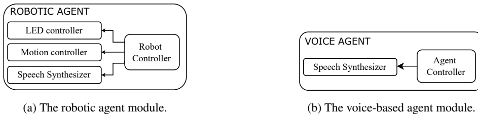
Figure 5: The agent module of REIT is implemented with a robotic agent and a voice-based agent for RoREIT and VoREIT, respectively.
