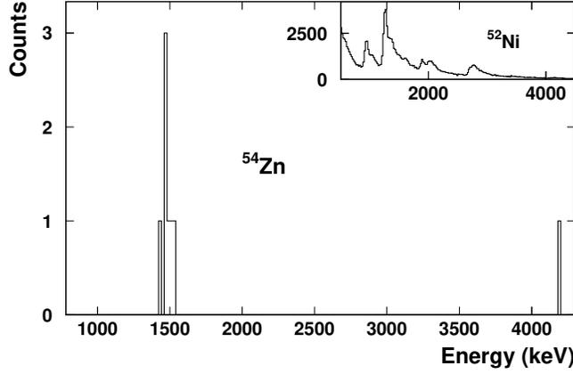
Figure 52: Decay energy spectrum measured for  $^{54}\text{Zn}$ . The peak at 1.48(2) MeV represents  $2p$  decay of this nucleus. The inset shows the decay energy spectrum for  $^{52}\text{Ni}$  dominated by  $\beta p$  decays. Reprinted with permission from Ref. [34]. Copyright (2005) by the American Physical Society.
