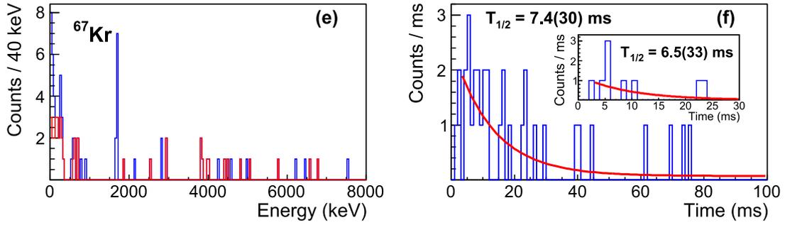
Figure 54: (Color online) Left: decay energy spectrum of  $^{67}\text{Kr}$ . The narrow peak at 1.69 MeV is due to  $2p$  radioactivity. Events shown in red were in coincidence with positrons detected in neighboring detectors. Right: Decay time distribution for  $^{67}\text{Kr}$ . In the inset the decay time for nine events in the 1.69 MeV peak is shown. Reprinted with permission from Ref. [36]. Copyright (2016) by the American Physical Society.
