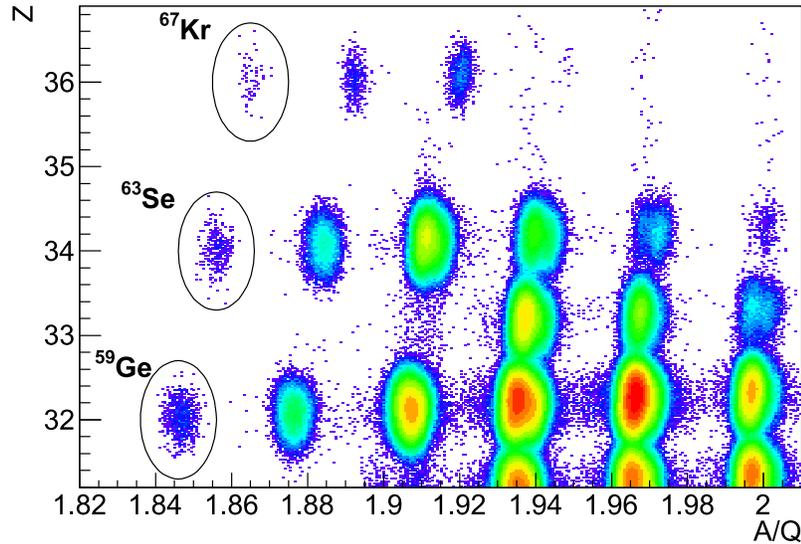
Figure 17: (Color online) Identification plot of atomic number  $Z$  versus the mass-to-charge ratio  $A/Q$  for ions selected by the BigRIPS separator at the RIKEN Nishina Center. The separator setting was optimized for  $^{65}\text{Br}$ . Reprinted with permission from Ref. [36]. Copyright (2016) by the American Physical Society.
