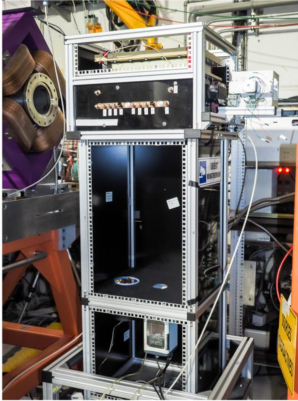
Figure 21: (Color online) The photograph of the Warsaw OTPC detector being mounted at the beamline, before installing the light-protecting closure. In the top part the active gaseous chamber is located. A CCD camera and a PMT can be seen at the bottom of the lower part.
