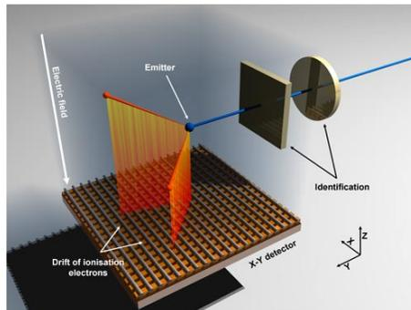
Figure 19: (Color online) Schematic illustration of the time-projection chamber operation principle. Reprinted with permission from Ref. [204]. Copyright (2007) by the American Physical Society.
