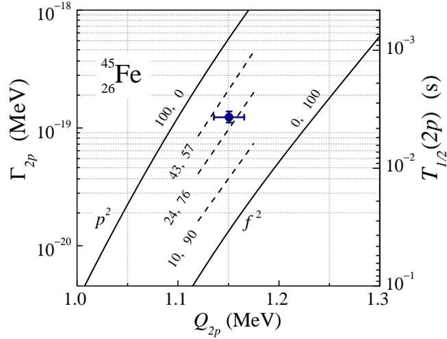
Figure 49: The partial  $2p$  half-life of  $^{45}\text{Fe}$  as a function of the  $2p$  decay energy. The experimental result is shown together with predictions of the 3-body model [72]. The decay width is taken from Ref. [73] and the decay energy from Ref. [243]. The numerical labels indicate the relative weights of the  $p^2$  and  $f^2$  configurations, respectively. Reprinted with permission from Ref. [73]. Copyright (2007) by the American Physical Society.
