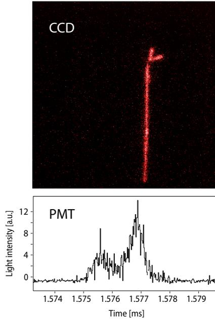
Figure 51: (Color online) An example of a  $2p$  decay event of  $^{48}\text{Ni}$  recorded by the Warsaw OTPC detector. Top: the image recorded by the CCD camera. A track of the  $^{48}\text{Ni}$  ion entering the chamber from below is seen. The two short tracks are protons emitted 1.576 ms after the implantation. Bottom: a part of the time profile of the total light intensity measured by the PMT showing in detail the  $2p$  emission.
