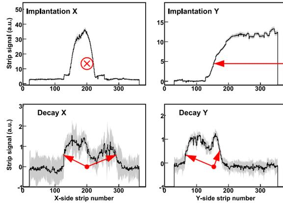
Figure 20: (Color online) One event of two-proton decay of  $^{45}\text{Fe}$  recorded by the Bordeaux TPC detector. The top row shows the implantation of a  $^{45}\text{Fe}$  ion. In the bottom the emission of two protons is seen from the point where the ion was stopped. Reprinted with permission from Ref. [204]. Copyright (2007) by the American Physical Society.
