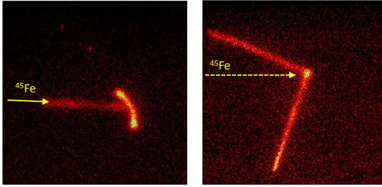
Figure 48: (Color online) Example CCD images of decays of  $^{45}\text{Fe}$  recorded by the OTPC detector in the experiment described in Refs. [73, 214]. Left:  $2p$  decay event, the track of a  $^{45}\text{Fe}$  ion entering the chamber from left is seen. Right:  $\beta 2p$  decay event, the track of the entering ion is not seen because the exposure of the camera was started just after implantation. Two long tracks represent delayed protons which escape the active detector volume.
