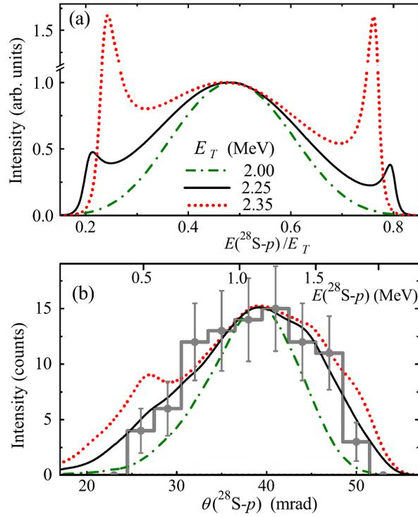
Figure 44: (Color online) (a) Transition from the direct  $2p$  decay to the sequential  $1p$ -emission mechanism: the proton spectra calculated by varying the  $2p$ -decay energy  $E_T$  of  $^{30}\text{Ar}$ . (b) The measured angular  $^{28}\text{S-p}$  correlations (histogram with statistical uncertainties) from the  $^{30}\text{Ar}$  ground state selected by choosing the gate (I) in Fig. 42(c) [190]. The data are compared with the respective MC simulations of the proton spectra in panel (a).
