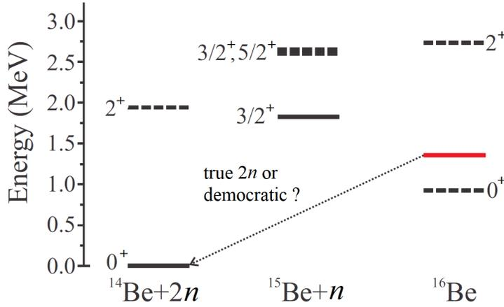
Figure 57: (Color online) The decay and level schemes of  $^{16}\text{Be}$  and  $^{15}\text{Be}$  isotopes derived in Ref. [256, 257]. The measured  $2n$  decay of  $^{16}\text{Be}$  ground state (red line) is shown by the dotted arrow. The vertical axis shows the decay energies with respect to the  $^{14}\text{Be}+2n$  threshold. The dashed black lines represent shell model calculations within the  $s$ - $p$ - $sd$ - $pf$  model space [256].
