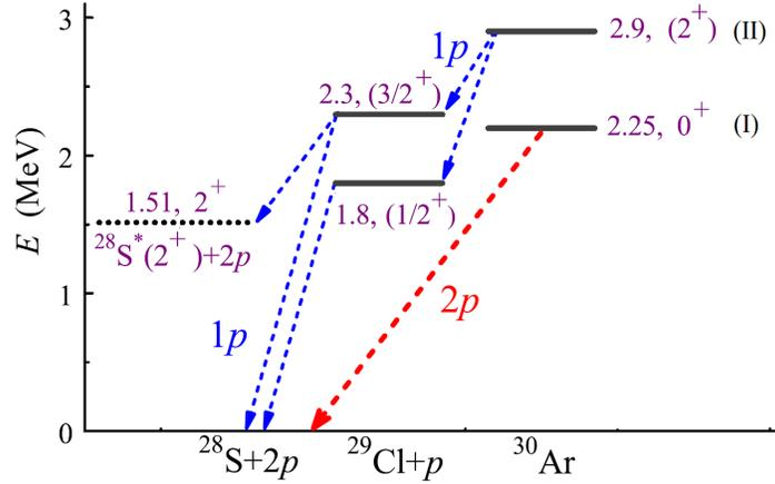
Figure 43: (Color online) Low-lying states and decay scheme of  $^{30}\text{Ar}$  derived in [190]. The assigned ground and first-excited states correspond to the peaks (I) and (II) in Fig. 42(c), respectively. The derived energies of states and tentative ( $J^\pi$ ) assignments are shown. Dashed arrow points to the g.s.  $2p$  decay, and short-dashed arrows indicate the assigned sequential proton emissions. The established intermediate resonances  $^{29}\text{Cl}$  are in the middle.
