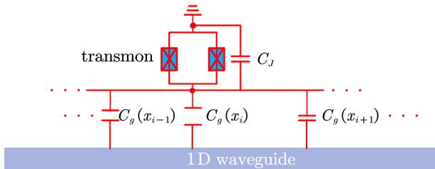
FIG. 3. Sketch of a feasible setup to realize our proposal: a transmon couples to a 1D coplanar waveguide at multiple coupling points via local capacitances  $C_g(x_i)$ . The real-space discretized coupling function is encoded into the capacitance sequence  $C_g(x_i)$ .
