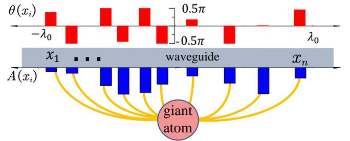
FIG. 1. (a) Sketch of our proposal: A giant atom couples to a conventional 1D waveguide at positions  $x_1, \dots, x_n$ . The coupling sequence  $g(x_i) = A(x_i)e^{i\theta(x_i)}$  is obtained via optimization methods.
